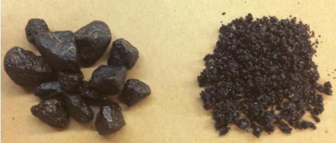
Figure 3-24 Separated coarse and fine particles for 50% RAP mixture
