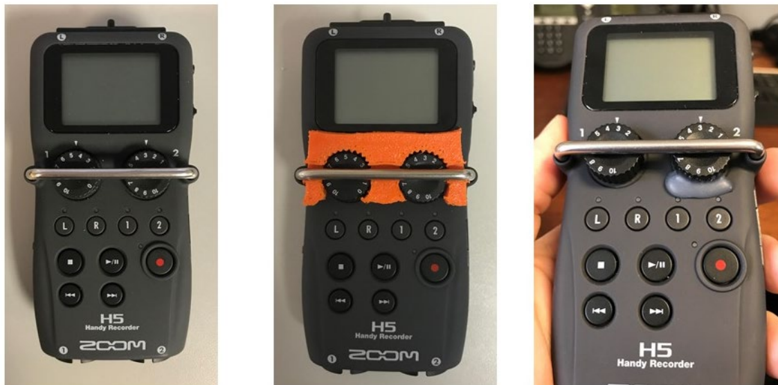
Figure 22: Sound recorder gain controller issues. The left pane shows two gain controllers behind a metal bar. As the protection of these controllers is minimal, the position of the controllers was changed in N=10 study participants after initial calibration. A 3D-printed gain control stabilizer (middle pane) was used for all remaining measurements. In the final approach, which will be used in the future National Sleep Study (but was not implemented around ATL), the gain controller was fixed in one position with a hot glue gun before calibration (right pane).
