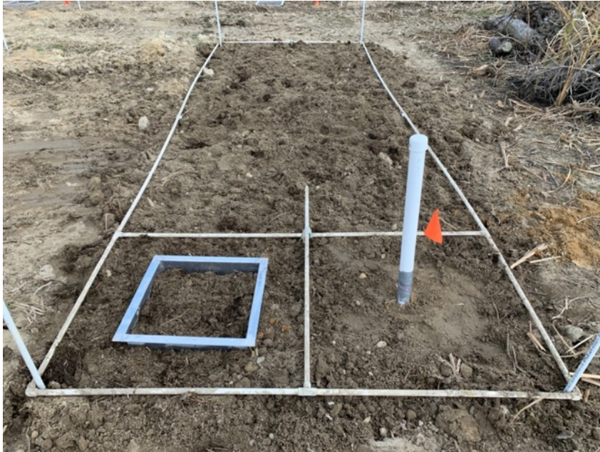
Photo 6 – Final Plot configuration . Metal rectangular structure is a gas chamber base. The aboveground pipe is a monitoring well. Dimensions are 2 meters x 6 meters.
