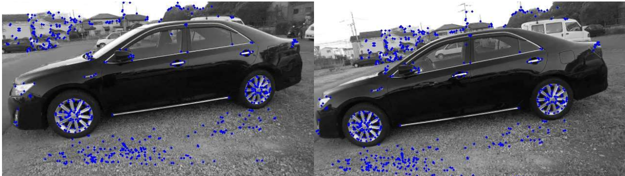
Figure 19. An illustration of the concept of keypoint identification (adopted from opencv.org). The blue points are keypoints identified in each image.
