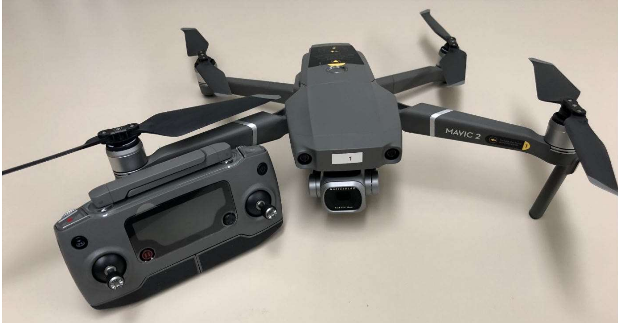
Figure 2. DJI Mavic Pro 2 UAV and onboard Hasselblad L1D-20c natural color digital camera.
