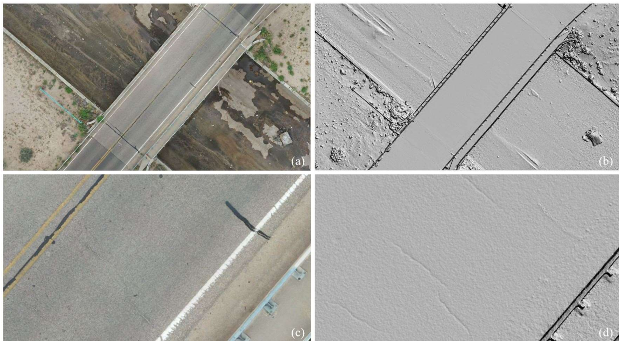
Figure 29. An illustration of the SfM products; (a) an overview of the orthophoto; (b) an overview of the DSM in shaded relief view; (c) a zoomed in view of the orthophoto; and (d) a zoomed in view of the DSM in shaded relief view.
