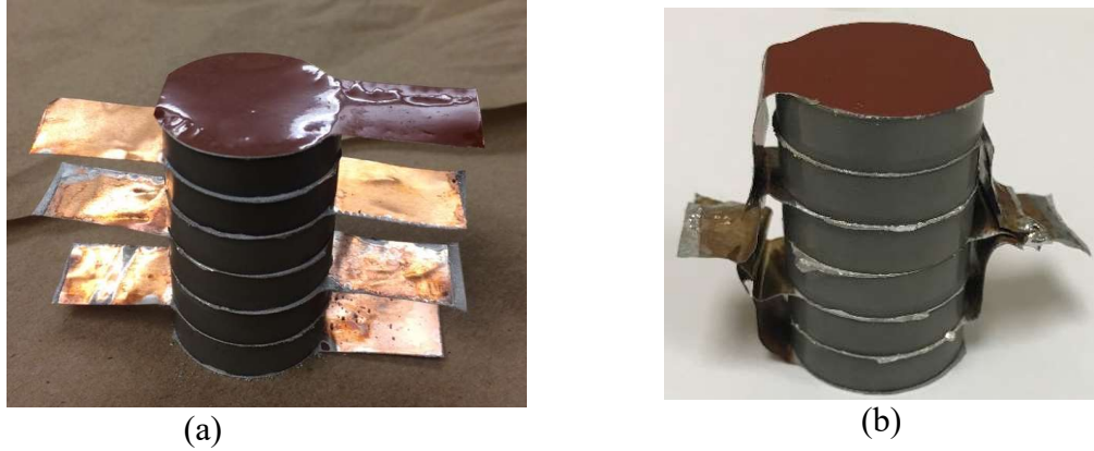
Figure 17. PEH elements (a) before soldering (b) after soldering.
