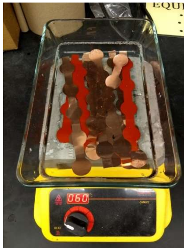
Figure 15. Work pieces resting in a 10% alkaline cleaner 60 °C tank.
