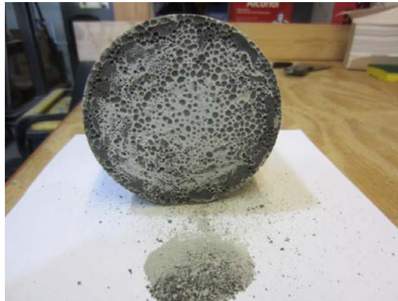
Figure 15. Photo. Grout sample scraped from the top layer of a cylindrical specimen of Product 3.
