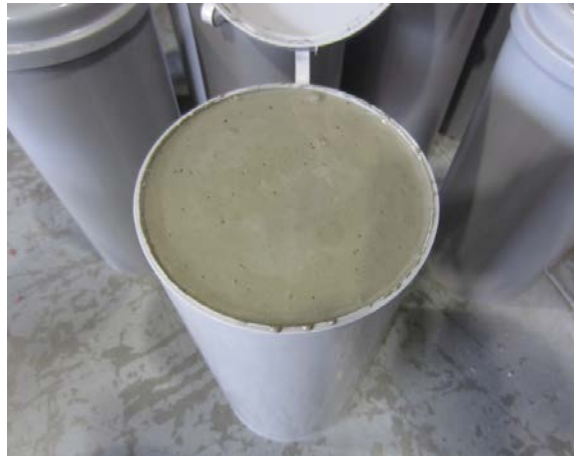
Figure 44. Photo. Fresh grout mix of a #2 Old Product 3 specimen made with the recommended water dosage.
