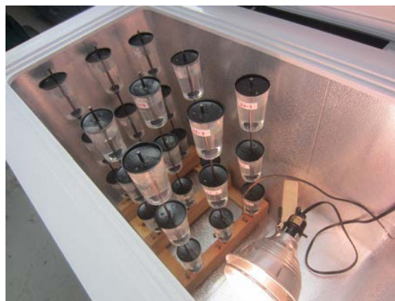
Figure 5. Photo. Elevated temperature test setup for Batch #2.
