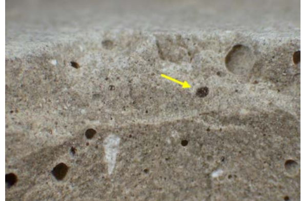
Figure 58. Photo. Sample #1 P3-2M at 15× magnification showing white particles and dark silica-fume agglomerates (arrow) on the fracture surface.
