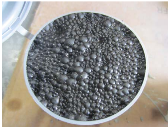
Figure 46. Photo. Fresh grout mix of a #2 Old Product 3 (opened bag) specimen made with the recommended water dosage.
