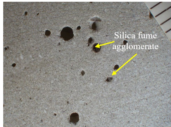
Figure 54. Photos. Middle and bottom slices from Sample #1 P3-2.
