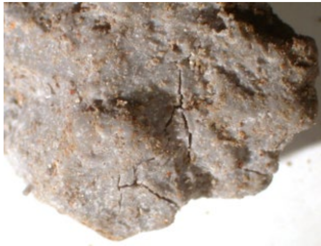
Figure 73. Photo. Field sample at approximately 10× magnification showing examples of desiccation cracks in air-dried soft grout.
