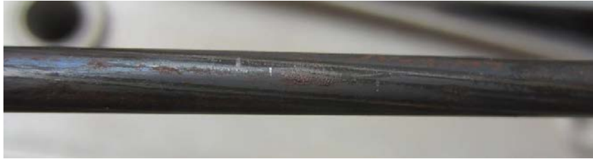
Figure 16. Photo. Close-up view of a center wire extracted from a Supplier A strand.
