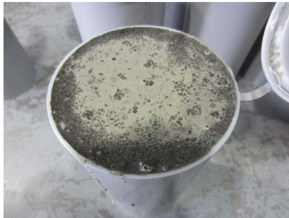
Figure 42. Photo. Fresh grout mix of a #1 Old Product 3 specimen.
