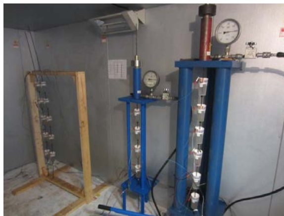
Figure 3. Photo. Cold temperature test setup (32 °F) for Batch #1 inside a walk-in environmental chamber.
