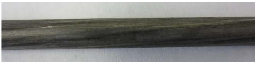
Figure 17. Photo. Close-up view of a center wire extracted from a Supplier B strand.
