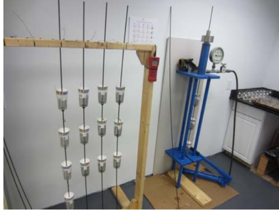
Figure 1. Photo. Ambient temperature test setup (77 °F) for Batch #1 with unstressed wires in the wooden frame and a stressed wire in the steel loading frame.
