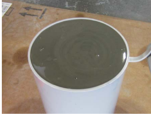
Figure 41. Photo. Fresh grout mix of a Product 1 specimen.
