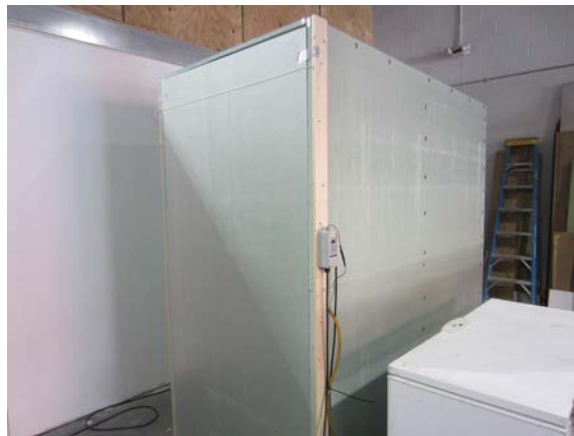
Figure 2. Photo. Elevated temperature test setup (104 °F) for Batch #1.
