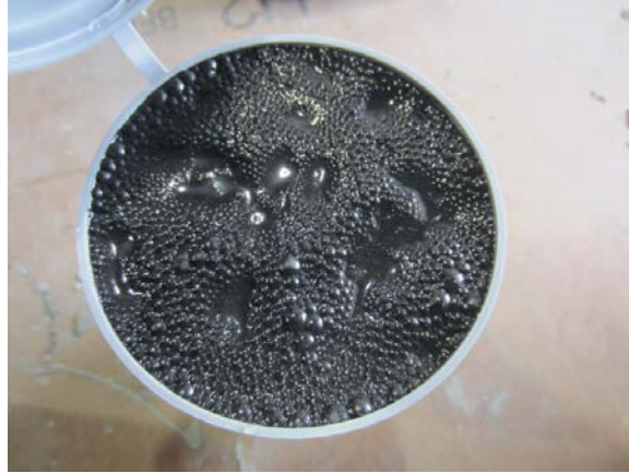
Figure 47. Photo. Fresh grout mix of another #2 Old Product 3 (opened bag) specimen after adding 0.5 lb of extra water to the fresh mix shown in figure 46.
