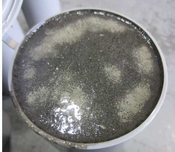
Figure 43. Photo. Fresh grout mix of another #1 Old Product 3 specimen after adding 0.5 lb of extra water to the fresh mix shown in figure 42.
