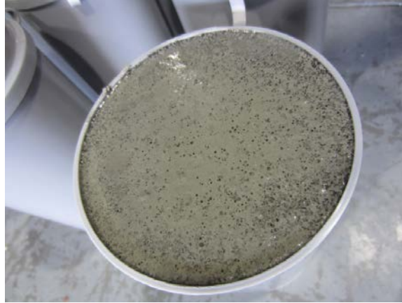
Figure 45. Photo. Fresh grout mix of another #2 Old Product 3 specimen after adding 0.5 lb of extra water to the fresh mix shown in figure 44.
