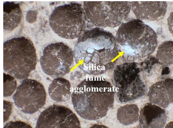
Figure 63. Photo. Sample #1 P3-4 xtra T at approximately 25× magnification showing ASR gel and silica-fume agglomerates in craters.
