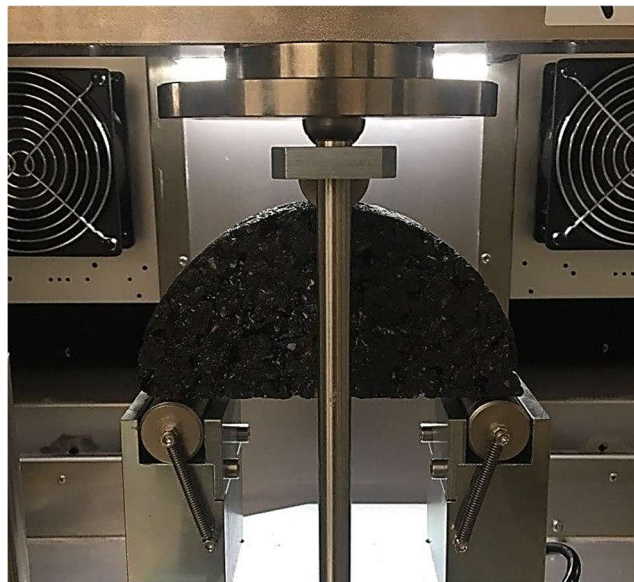
Figure 8. Set-up of Louisiana Semi-Circular Bending (SCB) test.
