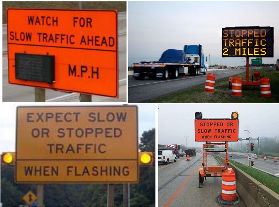
Figure 6. Examples of typical queue warning systems (QWSs) (34, 35).
