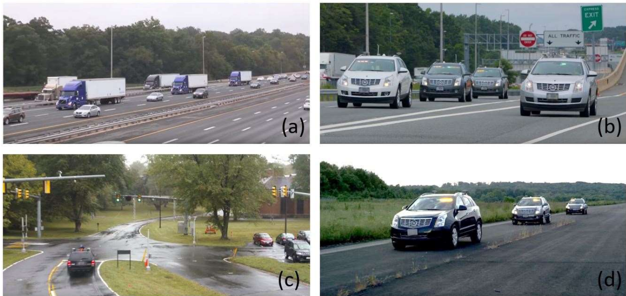
Figure 3. Examples of CAV applications with low automation levels: (a) truck platooning (11), (b) cooperative merging (12), (c) signalized intersection approach and departure (13), and (d) CACC (14).
