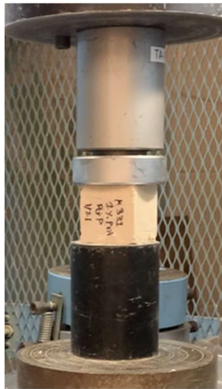
Figure 8. Compressive strength test experimental setup.
