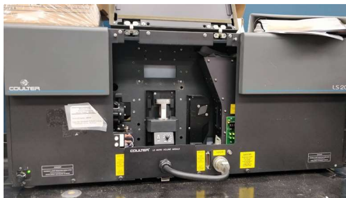
Figure 8. Beckman Coulter LS 200 for particle size analysis.
