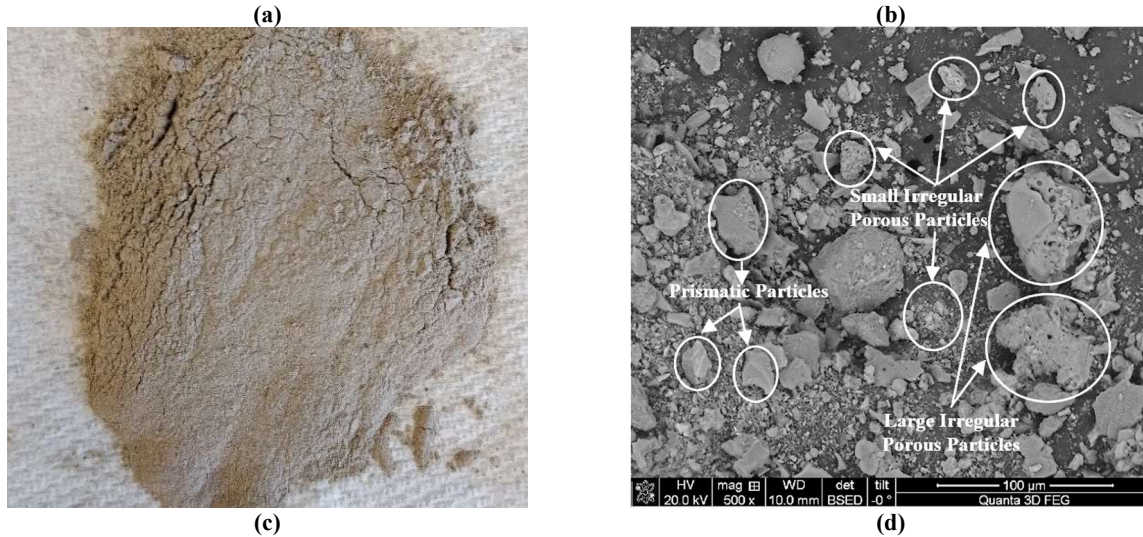
Figure 21. SCBAs' characterization (a) RBA (b) BSE-SEM image of RBA (c) PBA (d) BSE-SEM image of PBA
