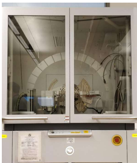
Figure 9. Panalytical Empyrean X-ray Diffractometer for XRD analysis.
