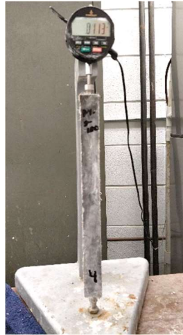
Figure 16. Digital length comparator with the test specimen.
