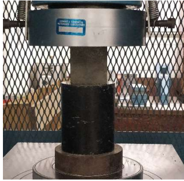
Figure 11. Compressive strength testing setup for 50.8-mm (2-in) mortar cubes.
