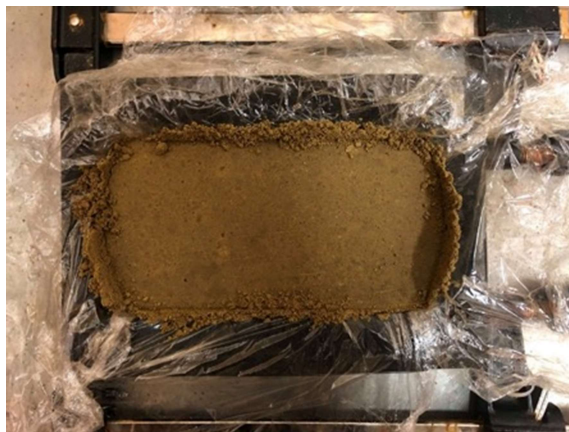
Figure A6. Specimen surface after removing the collar and wooden piece.
