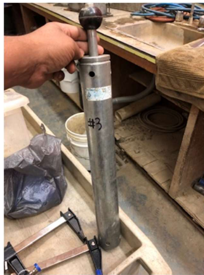
Figure A4. The 5.5 lb. manual rammer used during compaction.
