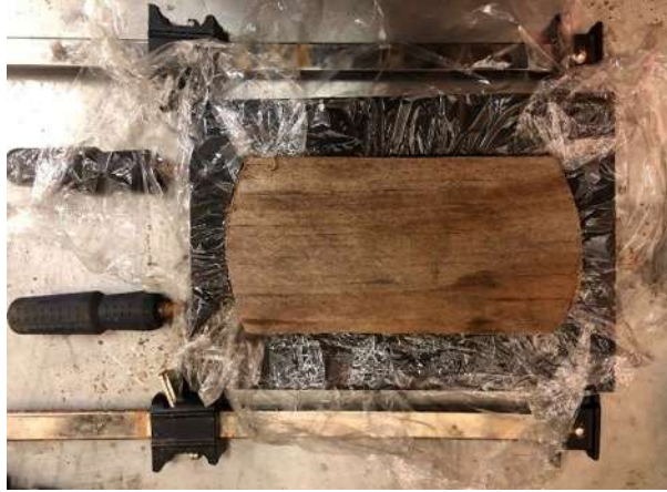
Figure A5. Placement of a wooden piece to facilitate compaction.
