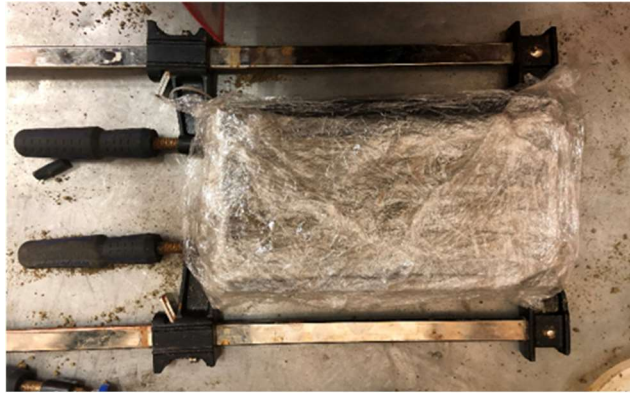
Figure A7. Wrapping the top surface of the specimen using plastic wraps.
