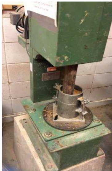
Figure 16. Compaction of soil with 5.5 lb. automatic rammer in 1/30 ft 3 cylindrical mold.
