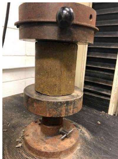
Figure 19. Determination of compressive strength of the soil-cement specimen in accordance with DOTD TR 432.
