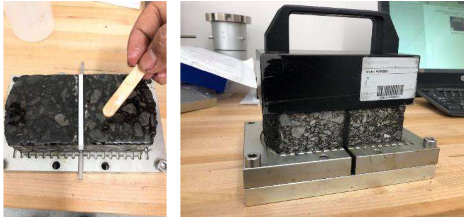
Figure 28. Gluing and curing of OT specimen: (a) spreading epoxy, and (b) curing of epoxy overnight.
