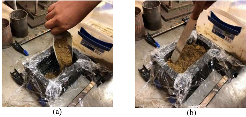
Figure A3. Pouring soil inside the mold using a scoop and spreading it evenly using a spatula.
