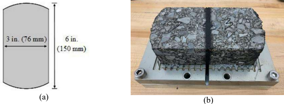
Figure 11. Upgraded TTI OT specimen, (a) with a smaller size (6 in. diameter), and (b) mounted on the base plates before testing.
