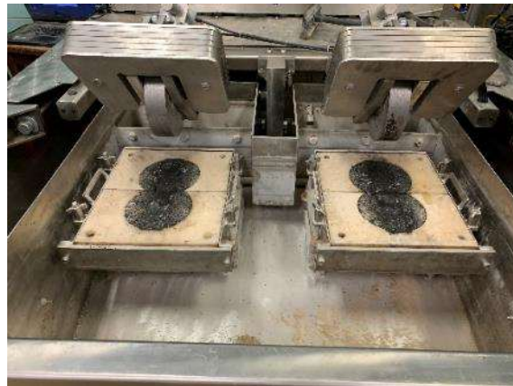
Figure 7. Hamburg Wheel Tracking Tester (HWTT) device.
