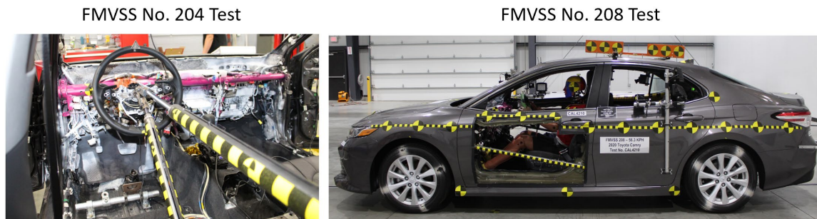
Figure 25. Full-Scale Tests (a) FMVSS No. 204; (b) FMVSS No. 208
