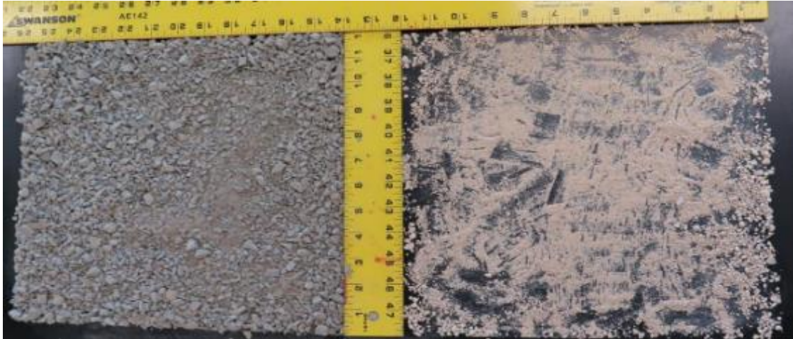
Figure 2. Micro-Surface (left) versus UTSS (right) Aggregate Rates.
