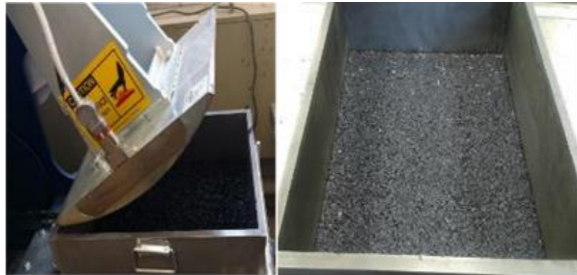
Preparing HMA slabs using the ARC compactor
