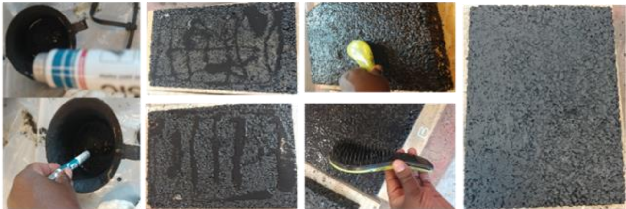
Preparing HMA slabs using the ARC compactor
