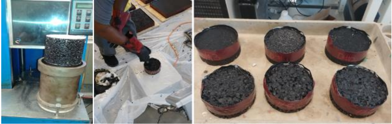
Figure 15. UTSS Treatment Application on Type D and PFC Molds.
