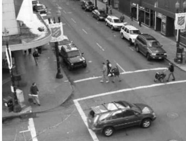
Figure 1. Many people who use crosswalks are traveling at different speeds. Pedestrian walking speeds generally range between 0.8 to 1.8 meters/second (2.5 to 6.0 feet/second).
