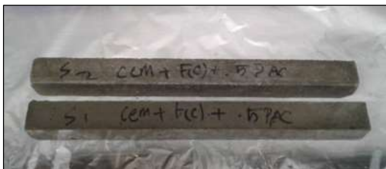
Figure 13. Mortar Bars Prepared for the Scaling Resistance Tests.
