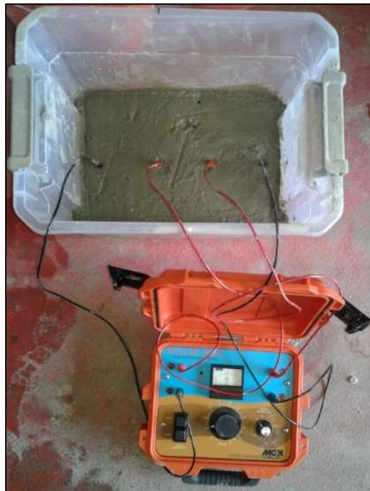
Figure 5. Schematic Set-up of Electrical Resistivity in the Laboratory.
