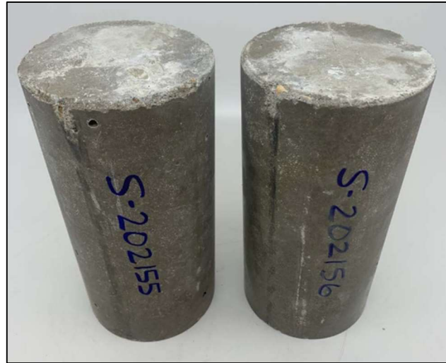
Figure 14. Samples Used for Determining the Air Content of Hardened Concrete.
