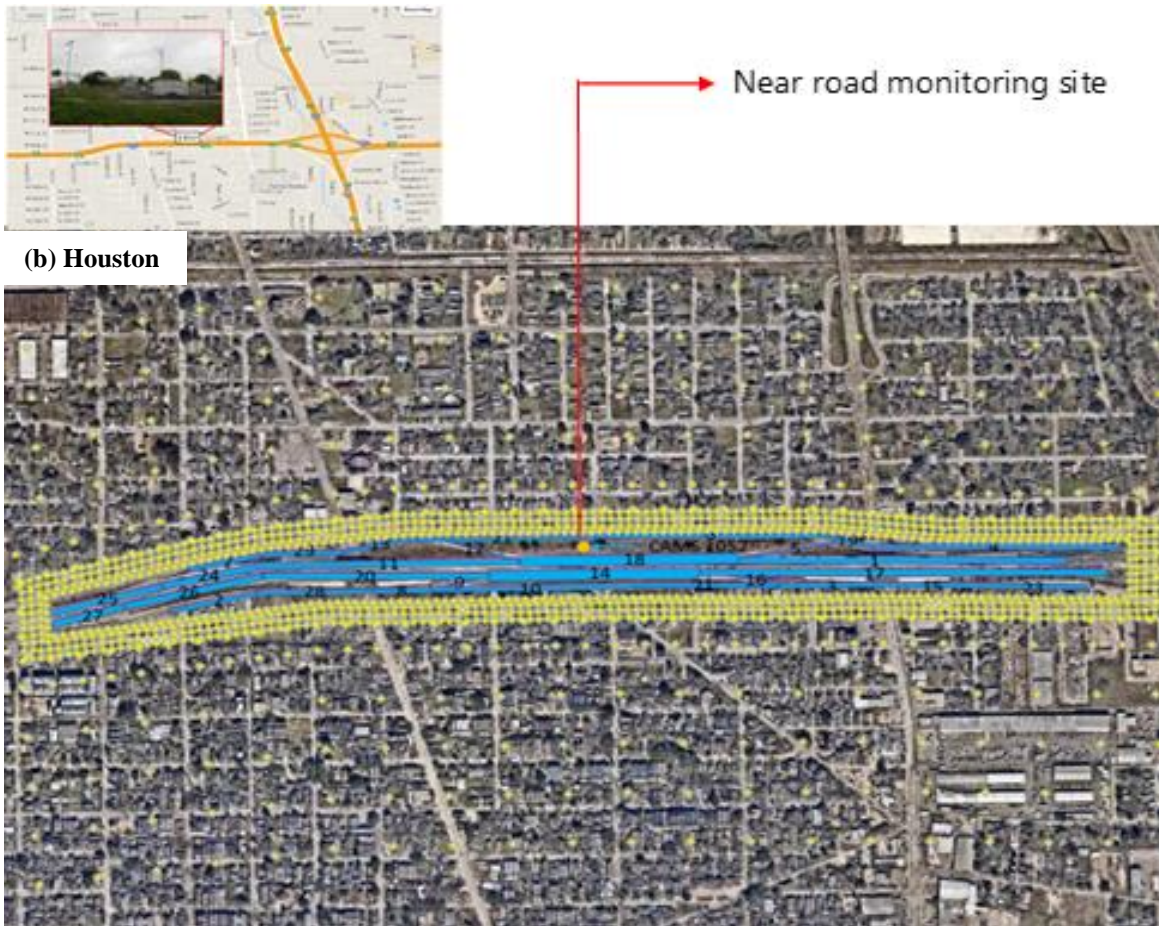
Figure 40. AERMOD Area Source and Receptor Placement for Houston Site.
