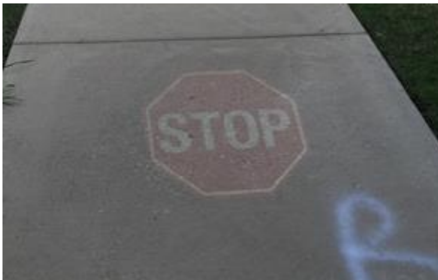
Figure 18. Projected Warning Sign.
