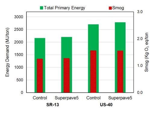
Figure 3. Environmental performance of materials used on SR 13 and U.S. 40.
