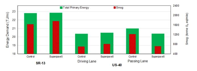
Figure 4. Environmental impacts associated with roughness on the SR 13 and U.S. 40 projects.
