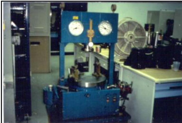
Figure 6. 1991, Rainhart Company, Modified Gyratory Shear Test Machine
