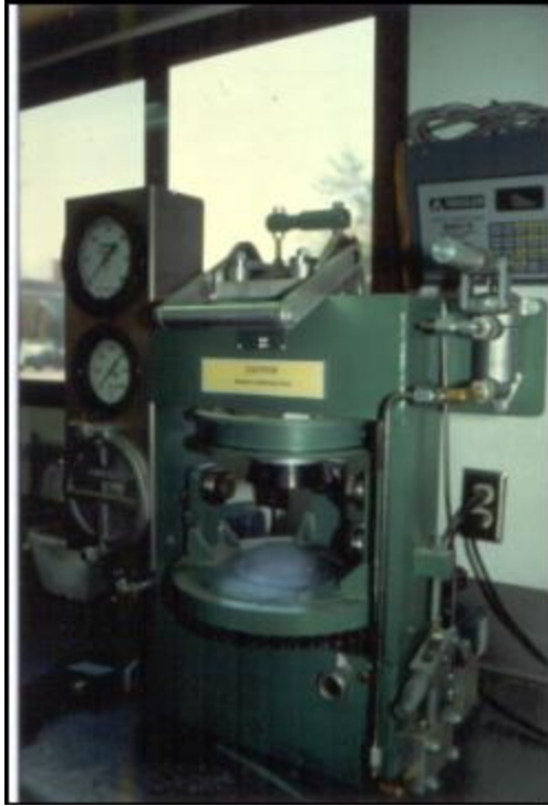
Figure 5. 1987, Rainhart Company, Gyratory Shear Test Machine
