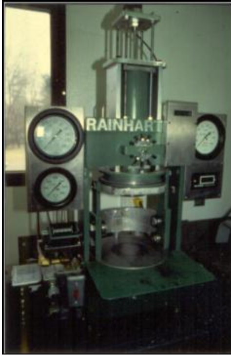
Figure 6. 1991, Rainhart Company, Modified Gyratory Shear Test Machine
