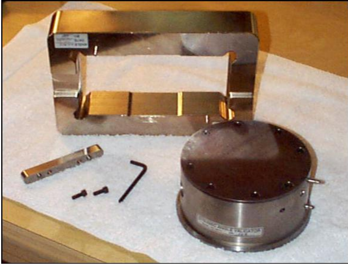
Figure 10. Test Quip AVK with NIST traceable verification fixture.
