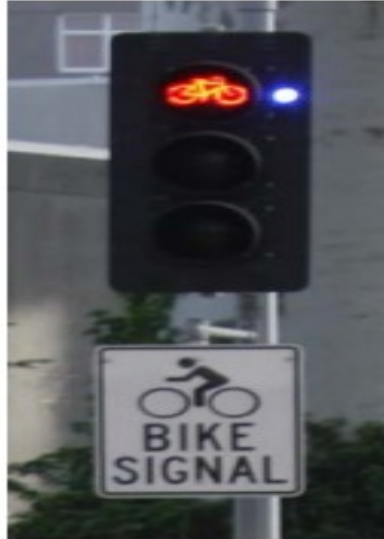
Figure 3.1: Blue detection confirmation light in backplate
