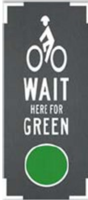
Figure 2.12: Modified Columbia experimental bicycle pavement marking (Wojciechowski, 2017)
