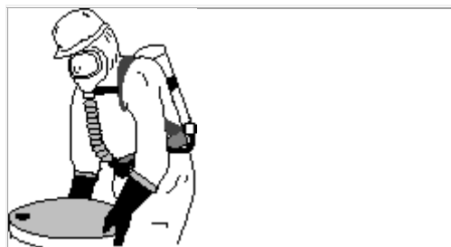
Figure 4-10. Self-contained breathing apparatus.
