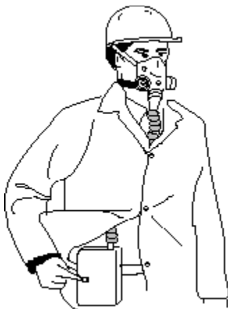
Figure 4-5. Powered air-purifying respirator.
