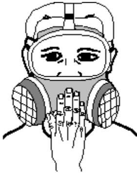
Figure 4-12. Positive pressure fit check.
