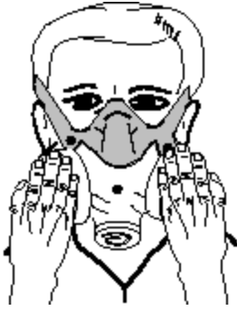
Figure 4-13. Negative pressure fit check.
