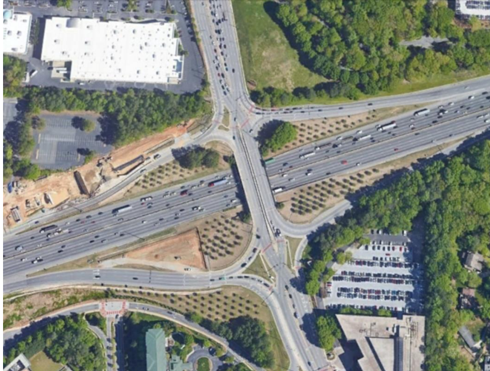
Figure 35. Photo. Aerial view of the DDI at I-285 and Ashford Dunwoody Rd. (Source: Google Earth)
