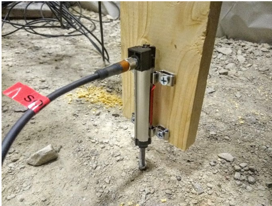
Figure 3-8: Photo of LVDT Located on GAB Layer
