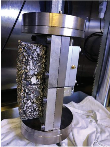
Figure 4.9 Setup of laboratory overlay test.
