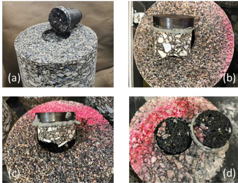
Figure 3.2 Photos of failed samples after pull-off testing: (a) HFST with scarification milling, (b) HFST with vacuum sweeping, (c) HFST with shot-blasting, and (d) chip seal pavement.
