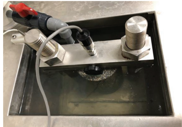
Figure 2.5 CTE test set-up.
