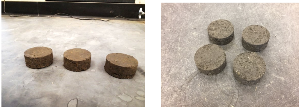
Figure 3.15 Compacted samples after cutting and trimming (Left: Glacial tills from Lincoln, Right: Weathered shales from Verdigre)
