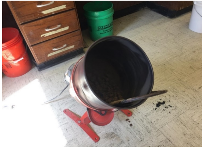
Figure 3.12 Mixing soil with biopolymers and water (Song et al., 2018)
