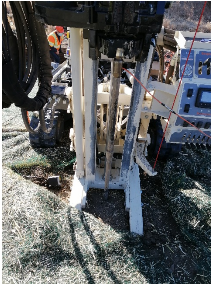
Figure 5.7 Scene of CPT(PCPT) testing
