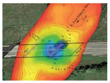
Figure 3. Hydrographic surveys indicated that water elevation upstream and downstream of this Nebraska Route 13 bridge near Hadar was 5 feet or less, but over 20 feet at the bridge. (Source: Nebraska Department of Transportation)
