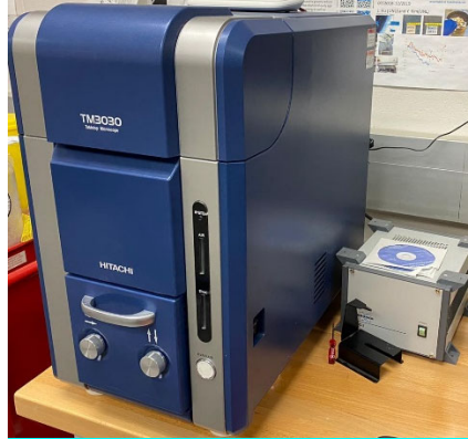
Figure 14. Hitachi TM3030 SEM and Quantax EDS unit.
