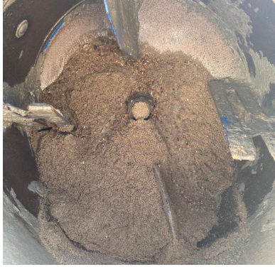
a) Loading of aggregate in the mixer
