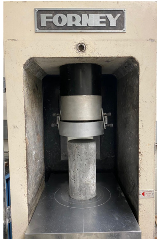
Figure 26. Compressive strength apparatus – Forney compression testing machine.
