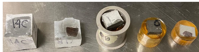
Figure 13. Microstructural analysis samples preparation procedure.
