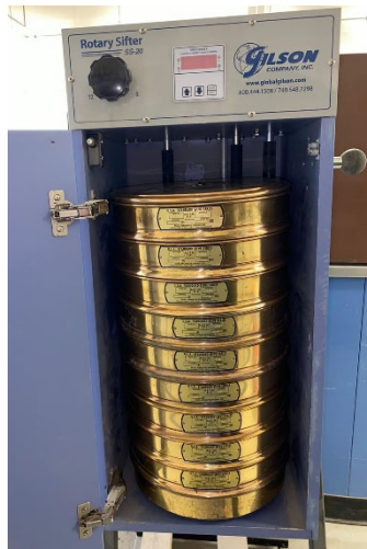
Figure 4. Aggregate sieve analysis setup.
