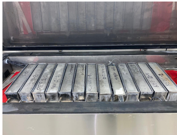
Figure 29. Freeze-thaw resistance testing apparatus.
