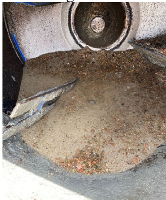
f) Clean aggregate covered with water
