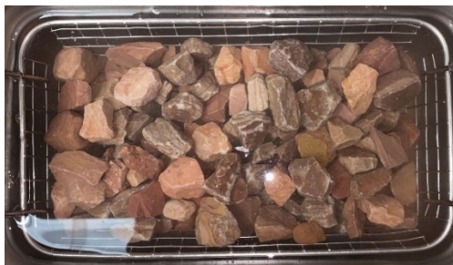
a) Aggregate immersed in an ultrasonic bath with clean deionized water
