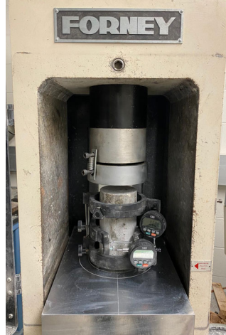
Figure 28. Modulus of Elasticity testing apparatus.
