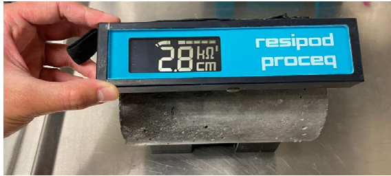
a) Surface resistivity measurement
