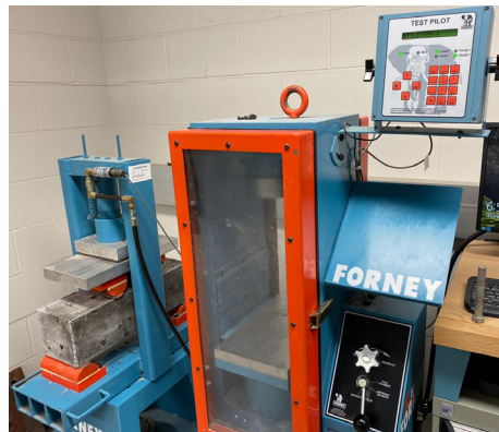
Figure 27. Flexural strength apparatus – Forney flexural testing machine.
