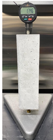
Figure 31. Free shrinkage test equipment setup.
