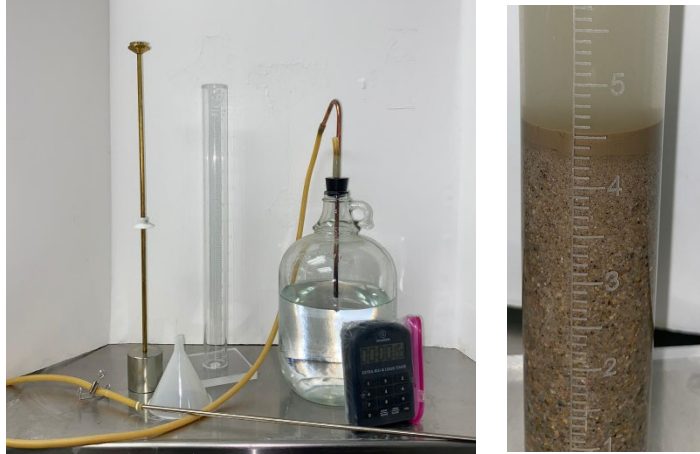
Figure 6. Sand Equivalent test apparatus and example of test result.
