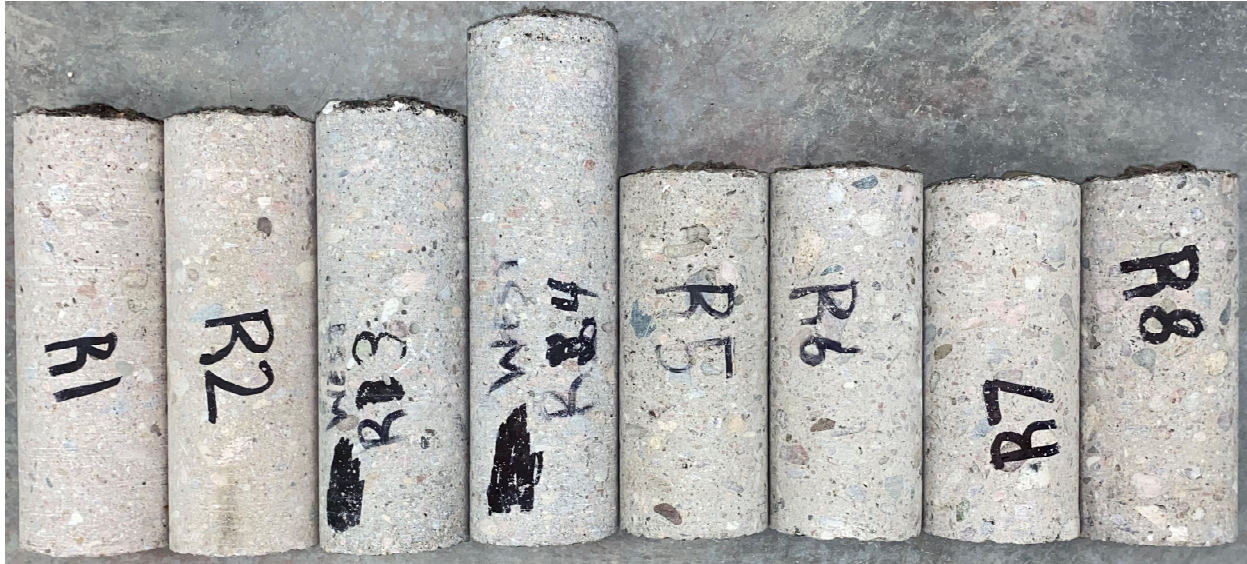
Figure 41. Core samples obtained from NDOT projects for inspection.
