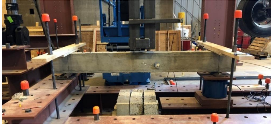
Figure 33. Photo. Anterior view of impact beam setup.
