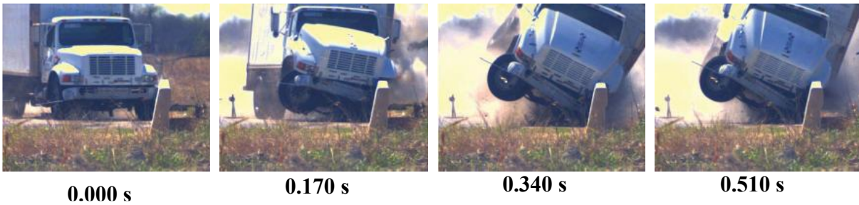
Figure 5. Photos. Typical single-unit truck impact response with single-slope barrier (Sheikh et al. 2012).
