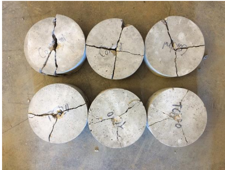
Figure 21. Photo. Fractured impact disk comparison: Control (top), 20.00 percent tire chip (bottom).
