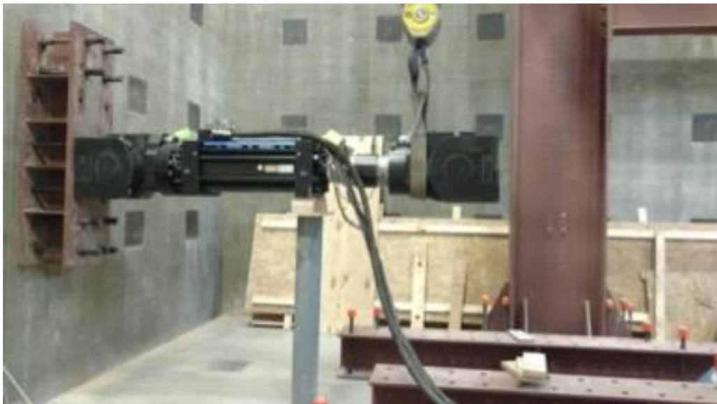
Figure 66. Photo. Actuator attached to strong wall.
