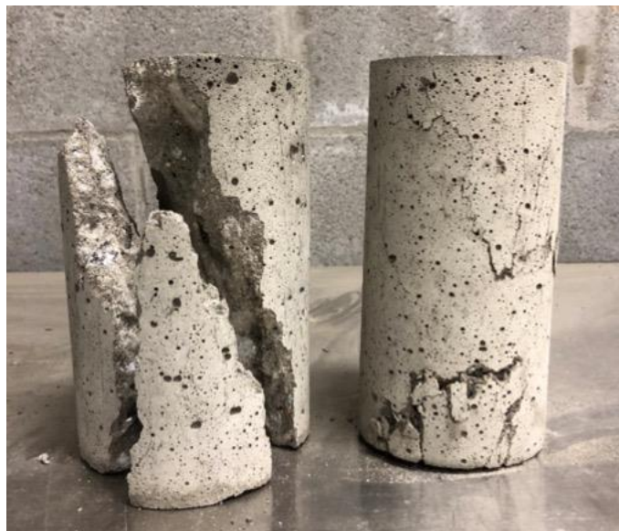
Figure 18. Photo. Comparison of compressive cylinders at failure: Control (left), rubberized steel fiber hybrid (right).
