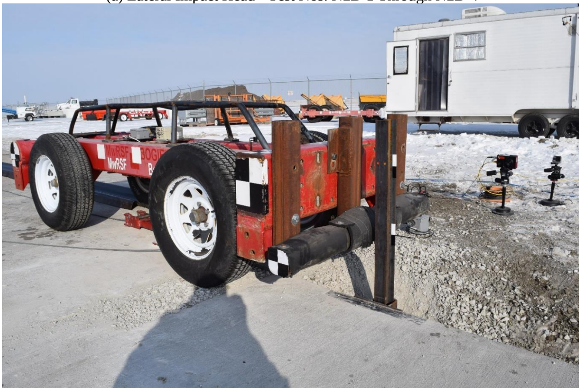
(b) Longitudinal Impact Head - Test Nos. N2B-5 and N2B-6
