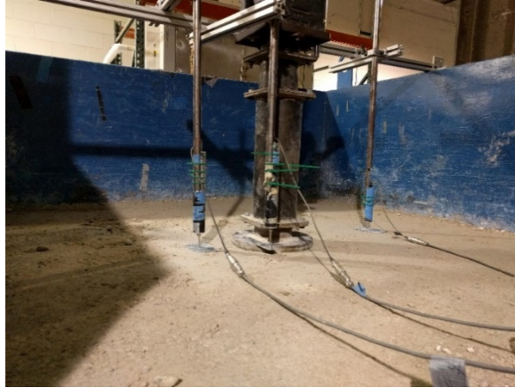
Figure 2.24: Displacement Transducers on the Surface of Base Course in An Unpaved Road Test
