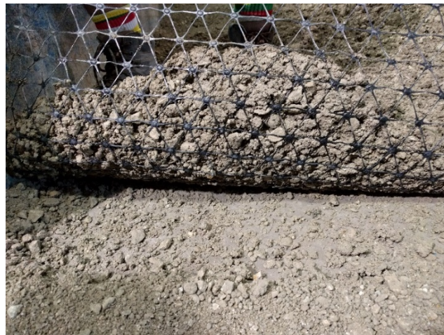
Figure 2.13: Triaxial Geogrid (with VGB)
