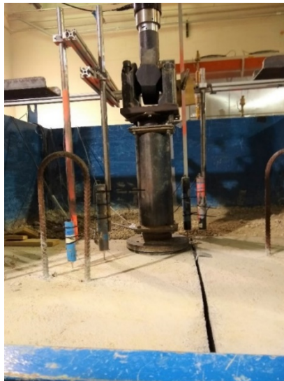
Figure 2.25: Displacement Transducers on a Concrete Slab in a Paved Road Test
