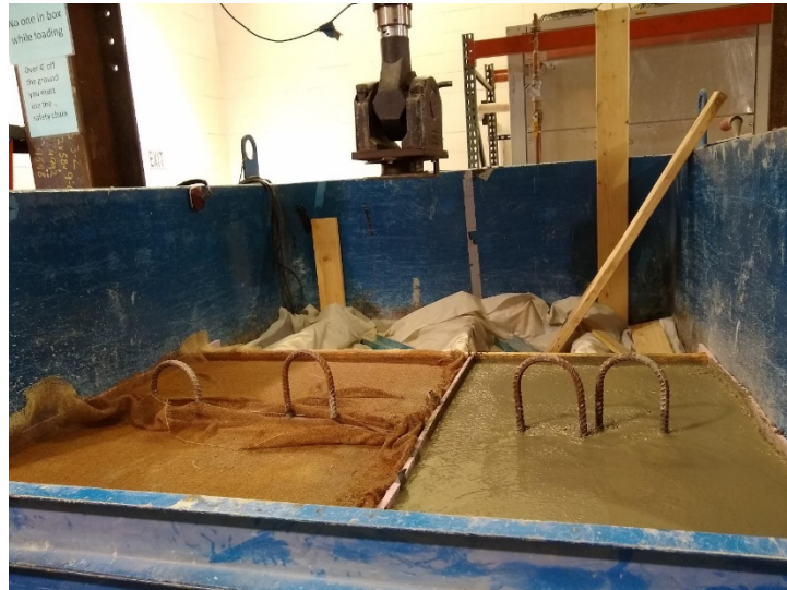
Figure 2.22: Concrete Slabs after Pour with An Overlying Burlap to Preserve Moisture
