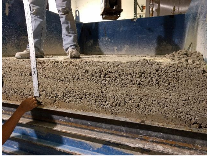
Figure 2.16: Direct Measurement of Base Course Thickness after the Test
