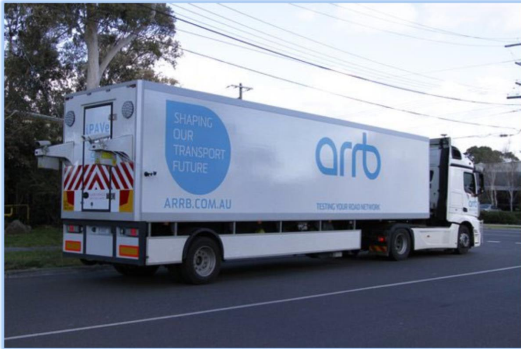
Figure 2-2 iPAVe used to collect pavement condition data in South Carolina (source: https://www.arrb.com.au/ipave ).
