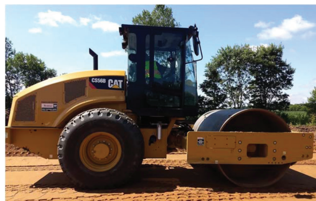
Figure 7.3 Caterpillar CS56B vibratory roller used for subgrade soil compaction.
