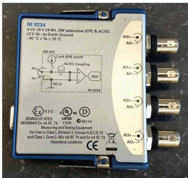
Figure 3.4 NI 9234 sound and vibration input module for collecting the signal from the accelerometer.
