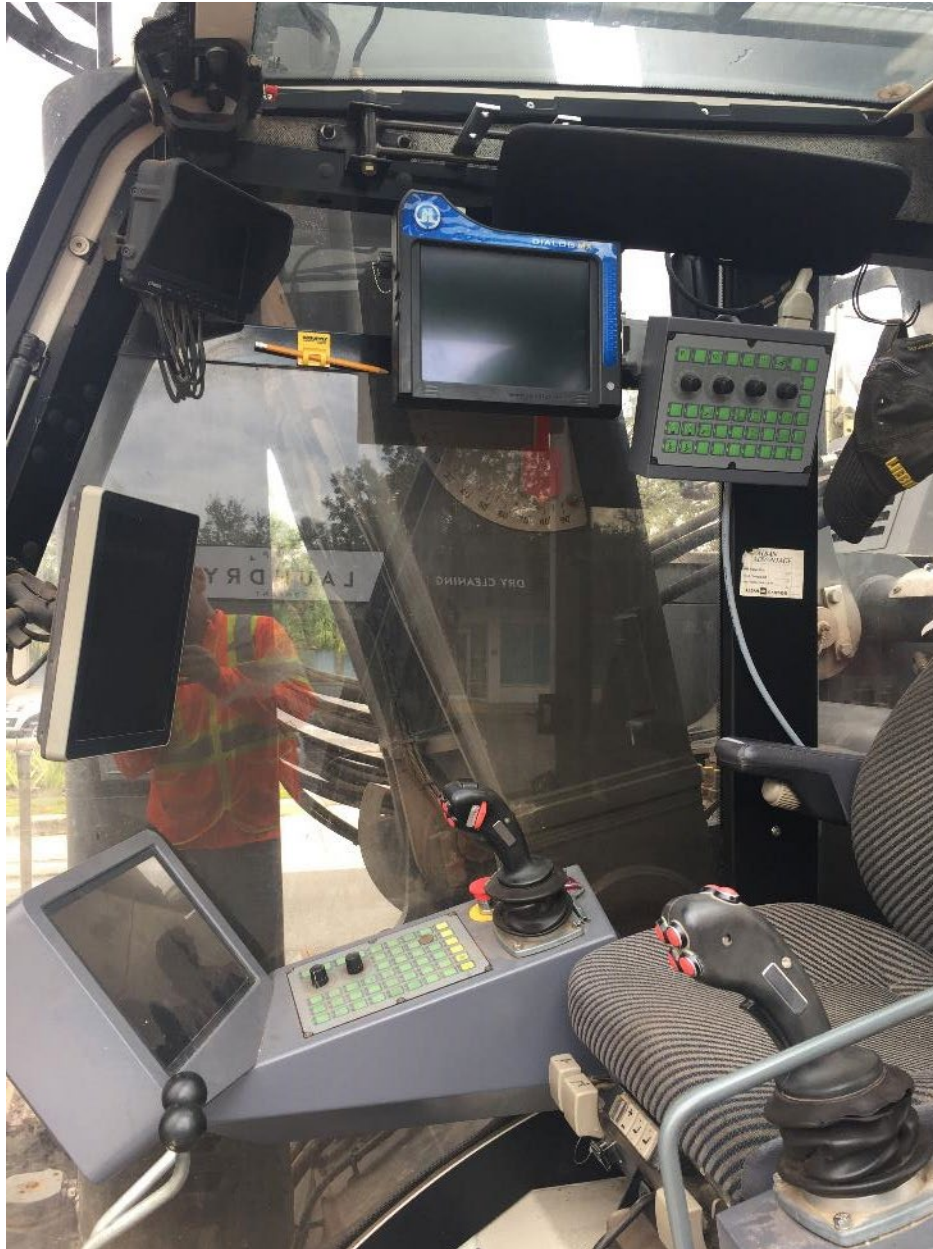
Figure 2-8. DIALOG mounted in the cab in a position that does not interfere with the driller.
