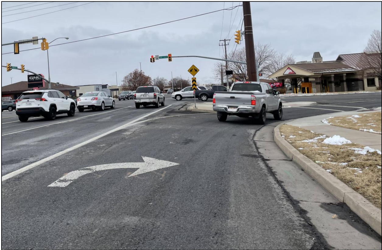
Figure 3-8 Channelized right-turn lane
