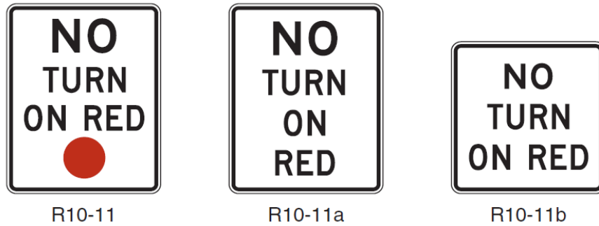
Figure 3-7 No-(right) turn-on-red signs (FHWA, 2009)
