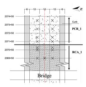
Figure 84. Plot. FWD test locations on top of HMA (east side of bridge).
