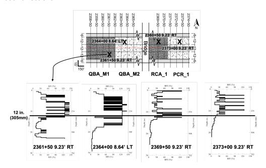
Figure 26. Graph. Sample DCP depth profiles on top of ASI capping layers.
