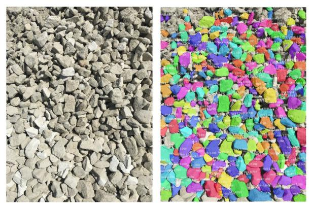
Figure 55. Photo. Raw and segmented images of QBA\_M2 section before compaction.
