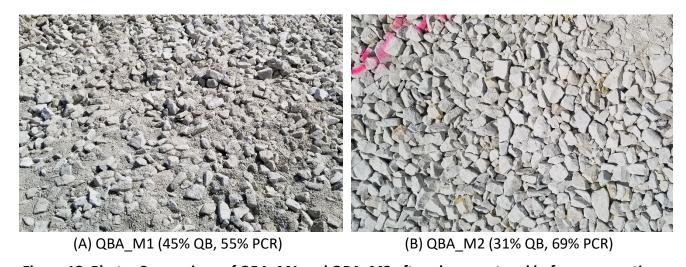
Figure 18. Photo. Comparison of QBA\_M1 and QBA\_M2 after placement and before compaction.
