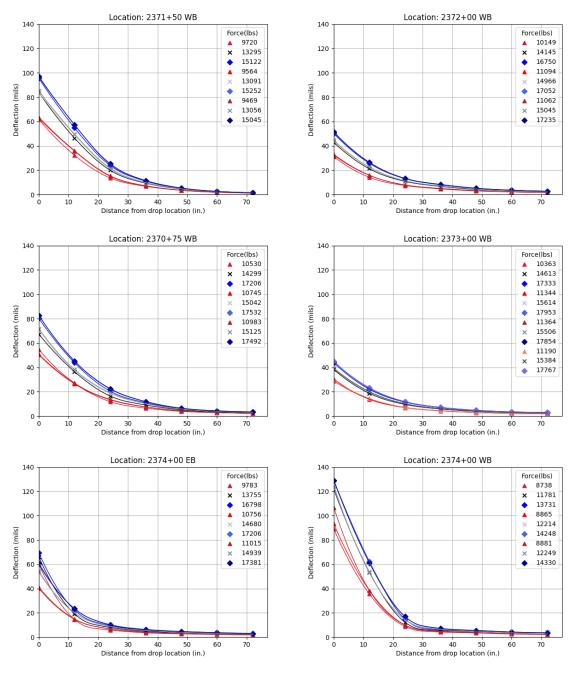
Figure 1. Graphs. FWD data on top of the capping layers at different measuring points in the conventional ASI sections.
