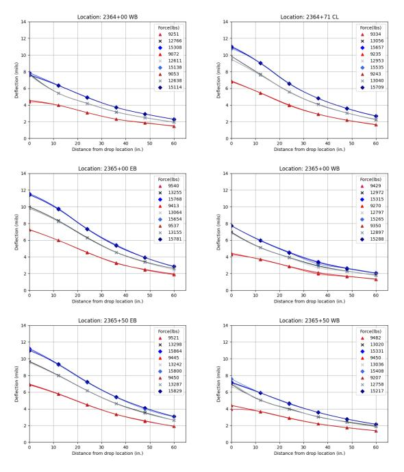
Figure 83. Graphs. FWD data on top of the HMA layer at different measuring points in the QBA sections (after opening to traffic).
