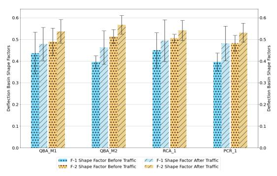
Figure 51. Chart. FWD deflection basin parameters (average values before and after traffic): shape factors F1 and F2.
