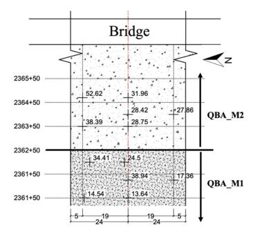
Figure 31. Plot. Composite surface moduli in MN/m<sup>2</sup> on top of QBA mixes, measured with LWD. (1 ksi = 6.89 MN/m<sup>2</sup>)
