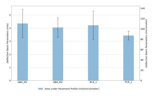
Figure 48. Chart. FWD deflection basin parameters (average values): Area under pavement profile.
