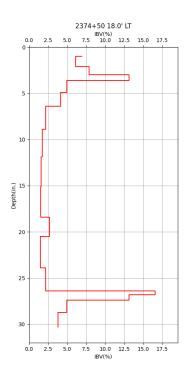
Figure 69. Graphs. DCP profiles of prepared subgrade at different measuring points (east side of bridge).
