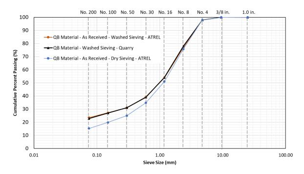
Figure 8. Graph. Grain size distribution of QB material (washed and dry gradations).
