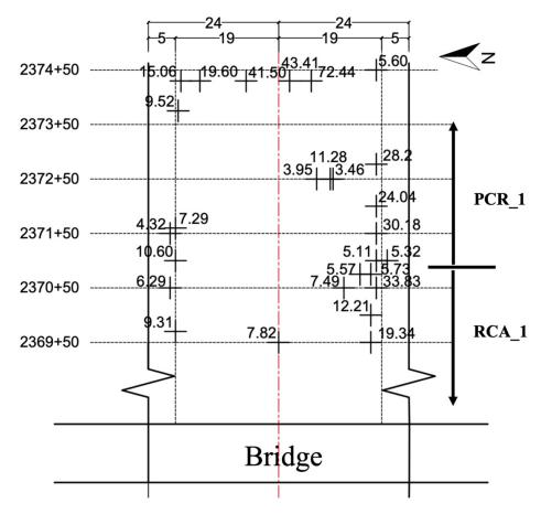
Figure 24. Plot. Achieved IBV(%) in the prepared natural subgrade (east side of bridge).
