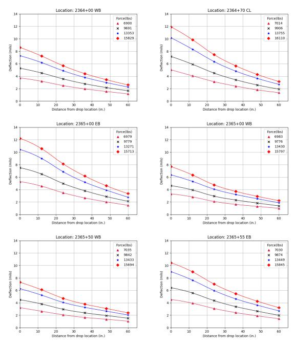
Figure 79. Graphs. FWD data on top of the HMA layer at different measuring points in the QBA sections (after construction).
