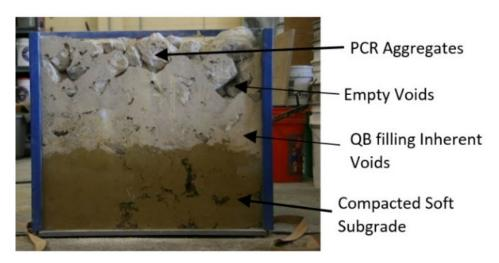
(B) Packing PCR and QB on top of weak (IBV = 1%) subgrade
