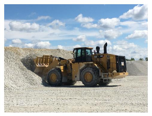
Figure 56. Photo. Scooping primary crushed rocks for blending at the quarry.
