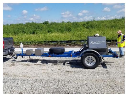
Figure 63. Photo. Conducting falling weight deflectometer testing on top of the capping layer of the PCR\_1 test section.
