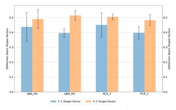
Figure 44. Chart. FWD deflection basin parameters (average values): shape factors F1 and F2.
