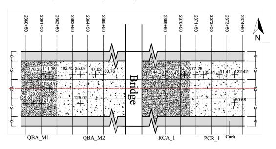
Figure 35. Plot. FWD surface deflections (mils) of center geophone ( $D_0$ ) on top of capping layer, normalized to a 12 kip (53 kN) load level.
