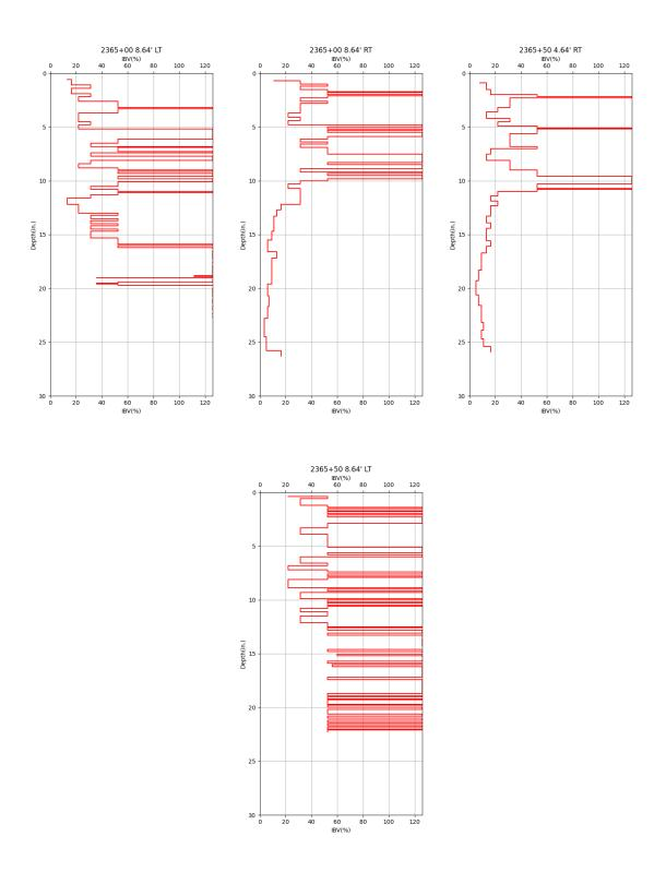
Figure 71. Graphs. IBV profiles from DCP tests on top of the capping layers (west side of bridge).
