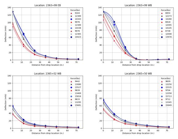
Figure 75. Graphs. FWD data on top of the capping layers at different measuring points in the QBA sections.
