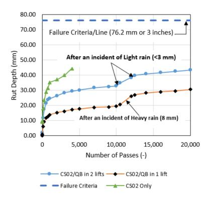
Figure 3. Graph. Rutting progression in the aggregate subgrade improvement layers with and without QB (test sections from ICT projects R27-168 and R27-124).
