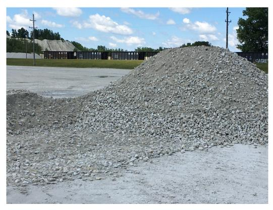
Figure 58. Photo. Blended stockpile for the QBA\_M1 material.
