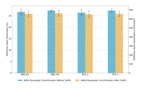
Figure 52. Chart. FWD deflection basin parameters (average values before and after traffic): AREA parameter.
