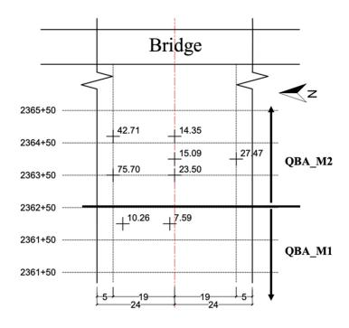
Figure 30. Plot. Subgrade moduli in  $MN/m^2$  measured with LWD for sections west of the bridge. (1 ksi = 6.89  $MN/m^2$ )
