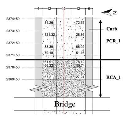
Figure 33. Plot. Composite surface moduli in  $MN/m^2$  on top of capping layer for conventional ASI sections on the east side of the bridge. (1 ksi = 6.89  $MN/m^2$ ).
