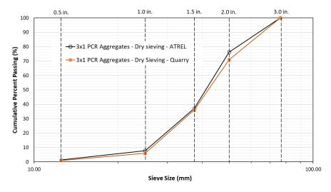
Figure 7. Graph. Grain size distribution of 3×1 PCR aggregates.
