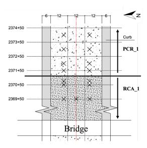
Figure 80. Plot. FWD test locations on top of HMA (east side of bridge).
