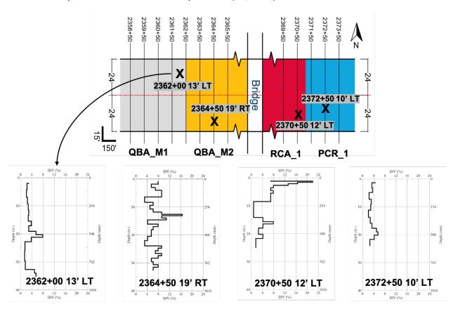
Figure 22. Graph. Sample DCP depth profiles for the prepared natural subgrade under all sections.
