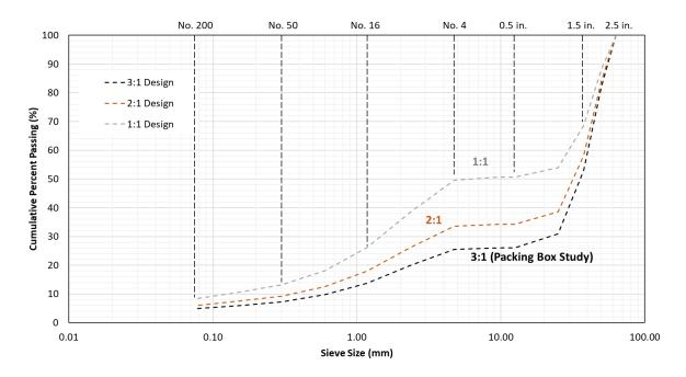
Figure 9. Graph. Proposed grain size distributions of different QBA mixes.
