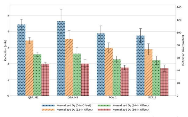
Figure 49. Chart. Recorded average FWD deflections for sensors D<sub>0</sub>−D<sub>3</sub> (after traffic).
