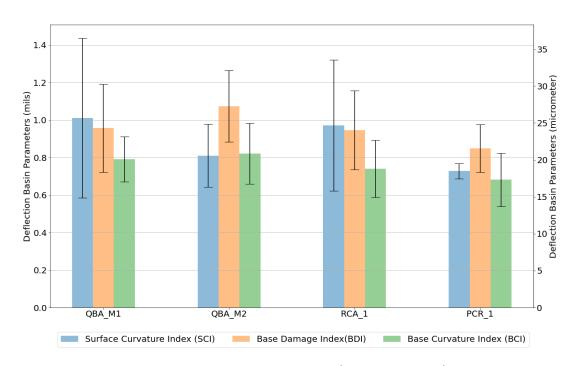
Figure 41. Chart. FWD deflection basin parameters (average values): SCI, BDI, and BCI.
