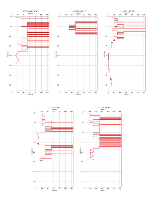
Figure 73. Graphs. IBV profiles from DCP test on top of capping layers (east side of bridge).
