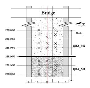
Figure 78. Plot. FWD test locations on top of HMA (west side of bridge).
