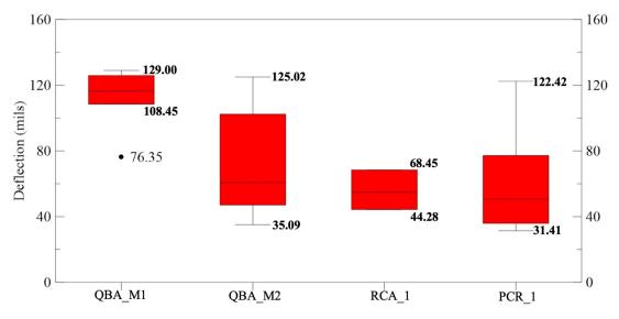
Figure 36. Diagram. Summary of FWD surface deflections (mils) of center geophone (D₀) on top of capping layer, normalized to a 12 kip (40 kN) load level.
