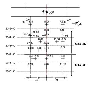
Figure 66. Plot. Achieved IBV(%) in the prepared natural subgrade (west side of bridge).
