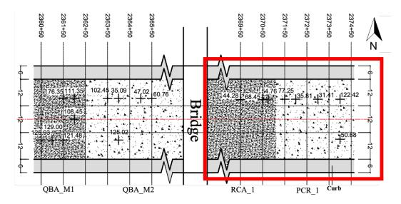
Figure 76. Plot. FWD average surface deflections (mils) of center geophone (D₀) on top of capping layer, normalized to a 12-kip (53-kN) load level.
