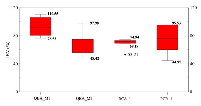
Figure 29. Diagram. Summary of average DCP (IBV) results for the different ASI layers.
