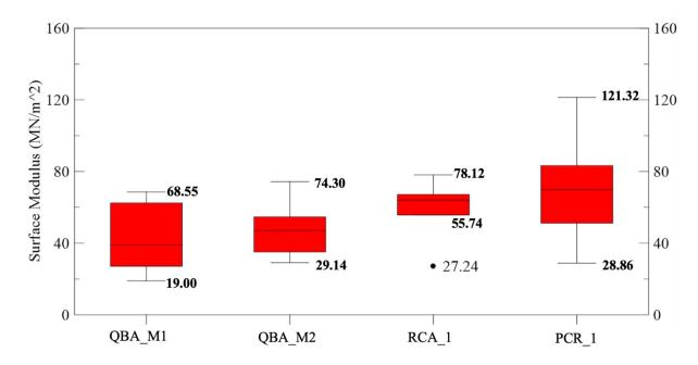
Figure 34. Diagram. Summary of LWD composite surface moduli on top of capping layers  $(1 \text{ ksi} = 6.89 \text{ MN/m}^2).$
