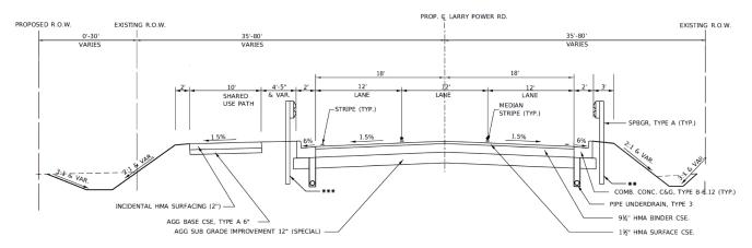
Figure 5. Illustration. Proposed Section 1 of Larry Power Road with 12 in. ASI (special)—
