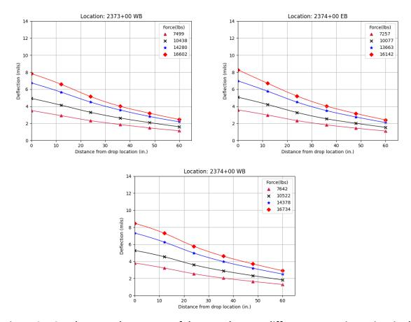
Figure 81. Graphs. FWD data on top of the HMA layer at different measuring points in the conventional ASI sections (after construction).
