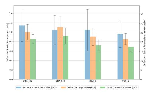
Figure 50. Chart. FWD deflection basin parameters after traffic (average values): SCI, BDI, and BCI.
