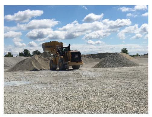
Figure 57. Photo. Weighing by-product sand in loader bucket to prepare quarry by-product aggregates.
