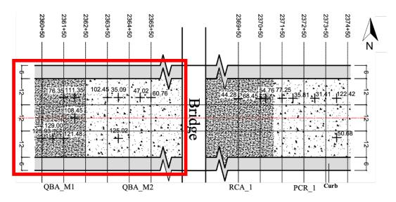
Figure 74. Plot. FWD average surface deflections (mils) of center geophone (D<sub>0</sub>) on top of capping layer, normalized to a 12-kip (53-kN) load level.
