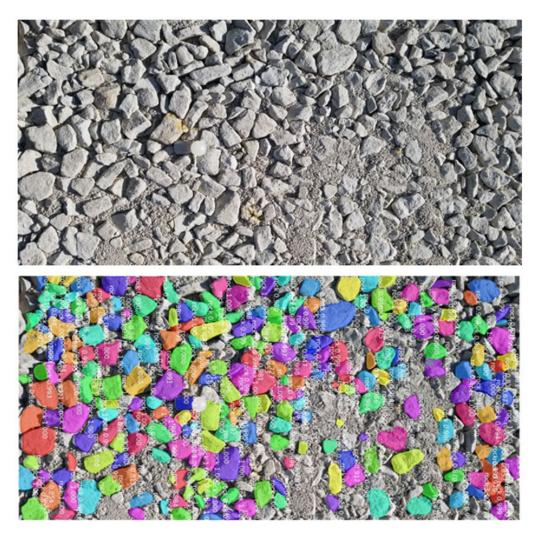
Figure 54. Photo. Raw and segmented images of QBA\_M1 section before compaction.
