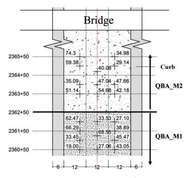
Figure 32. Plot. Composite surface moduli in  $MN/m^2$  on top of capping layer for QBA sections on the west side of the bridge. (1 ksi = 6.89  $MN/m^2$ ).
