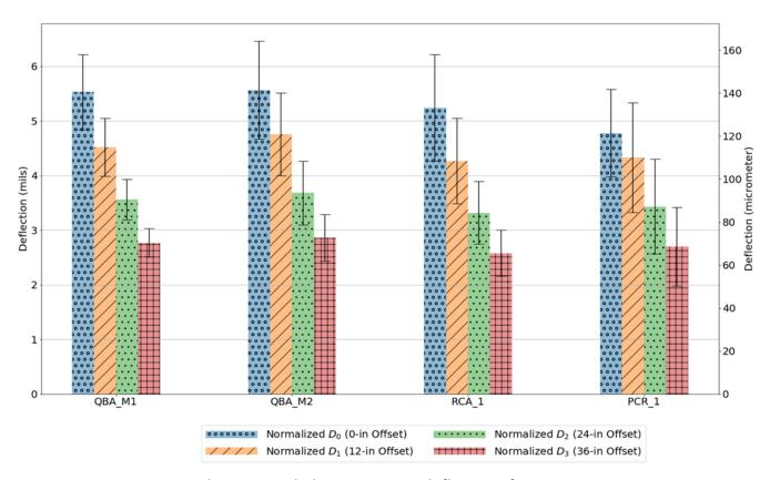
Figure 37. Chart. Recorded average FWD deflections for sensors D<sub>0</sub>-D<sub>3</sub>.
