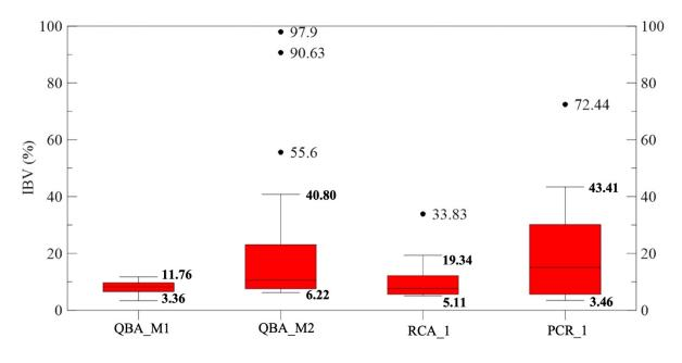
Figure 25. Diagram. Summary of average DCP (IBV) results for prepared natural subgrade.
