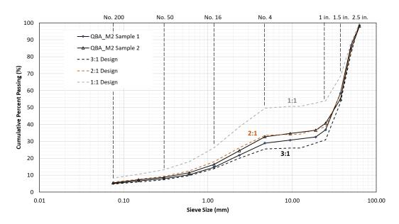
Figure 20. Graph. Grain size distributions of field samples collected from QBA M2 mix.
