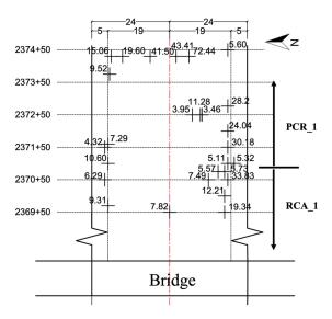
Figure 68. Plot. Achieved IBV(%) in the prepared natural subgrade (west side of bridge).
