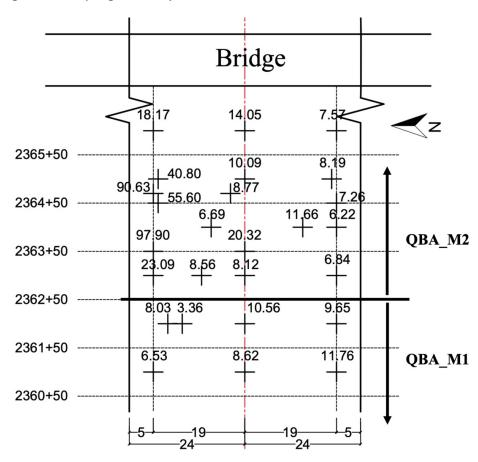
Figure 23. Plot. Achieved IBV(%) in the prepared natural subgrade (west side of bridge).
