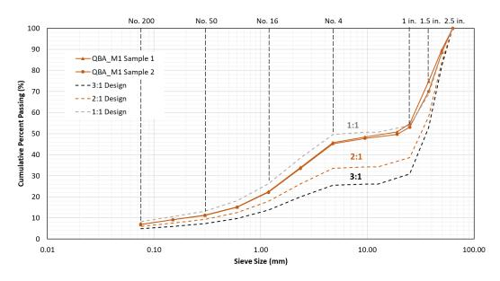
Figure 19. Graph. Grain size distributions of field samples collected from QBA M1 mix.
