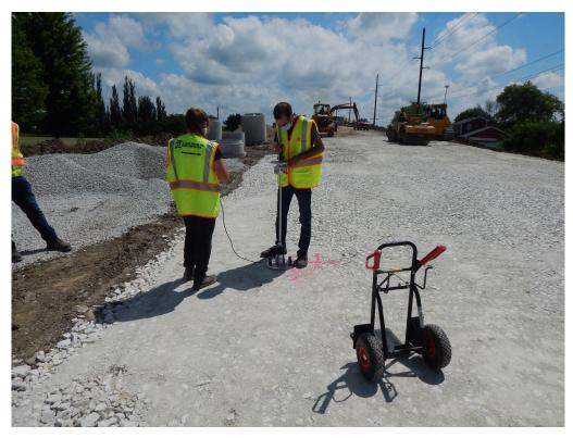
Figure 62. Photo. Conducting lightweight deflectometer testing on top of QBA\_M1 layer.
