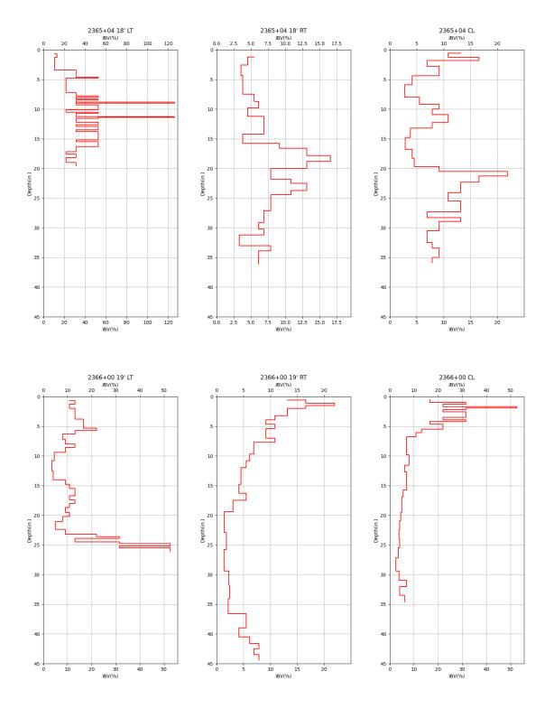
Figure 67. Graphs. DCP profiles for the prepared subgrade at different measuring points (west side of bridge).
