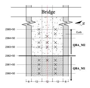
Figure 82. Plot. FWD test locations on top of HMA (west side of bridge).
