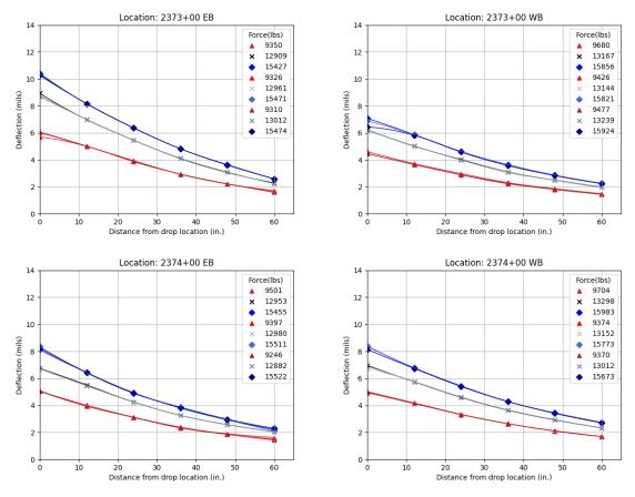
Figure 85. Graphs. FWD data on top of the HMA layer at different measuring points in the conventional ASI sections (after opening to traffic).
