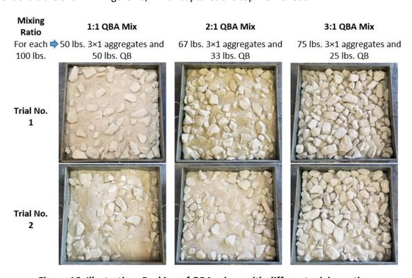
Figure 16. Illustration. Packing of QBA mixes with different mixing ratios.
