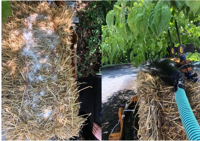
Figure 3. Straw Bale Treated With Granular H30 Polyacrylamide Flocculant (Left) and Dewatering Bag Test Conducted With the Addition of a Straw Bale Alone (Right)
