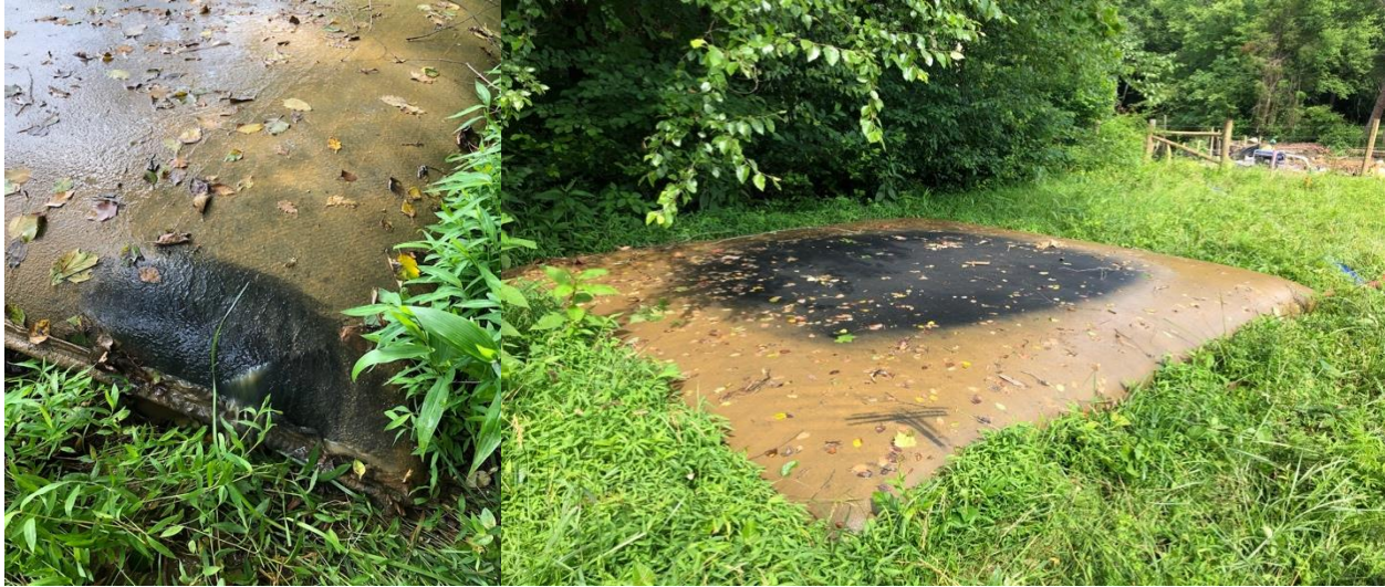
Figure 5. Field Observations From Site 3 Showing an Increase in Discharge From Areas of the Bag Where the Accumulated Filter Cake Was Disturbed During Sampling
