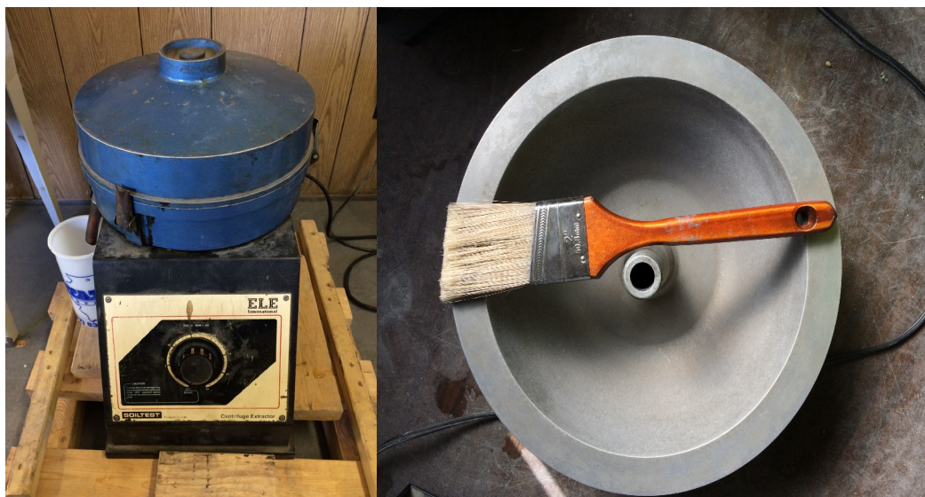
Figure 16. Centrifuge equipment and 3000 g bowl for spinning the FLWA to obtain surface moisture (Montanari et al. 2021).
