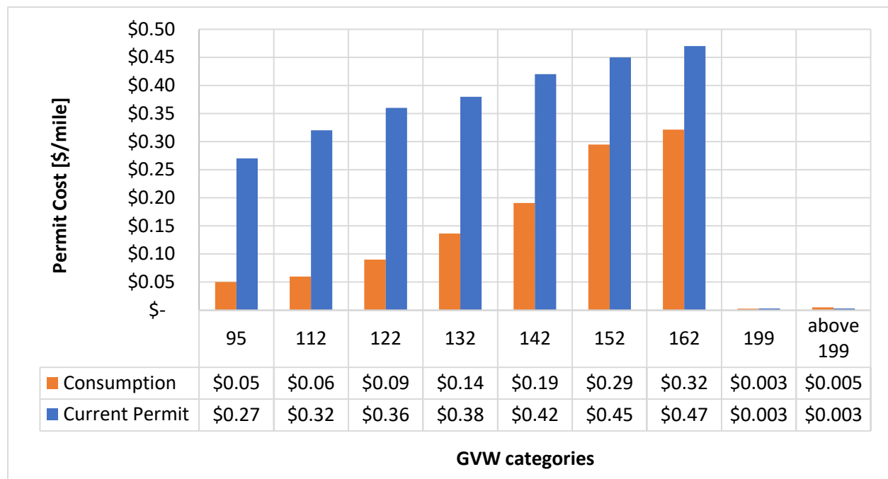
Figure 7-1. Bridge consumption for single trip permits vs. current permit fees in Florida.
