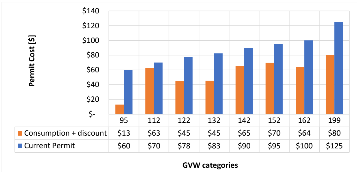
Figure 7-7. Bridge consumption for multi-trip 3-month permits with current discount vs. current permit fees in Florida.
