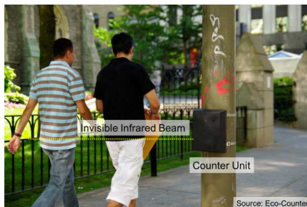
Figure 12: Passive Infrared Sensor for Counting Pedestrians and Bicyclists (ADOT).
