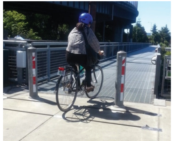
Figure 10: Bicyclist riding over pneumatic tubes (Source: Karla Kingsley, Kittelson & Associates, Inc. (Ryus et al., 2014b))
