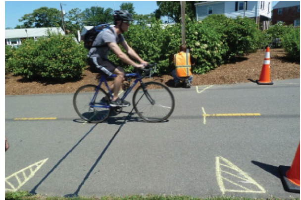
Figure 14: Bicyclist rising over piezoelectric strips. Source: Tony Hull, Toole Design Group (NCHRP 797).
