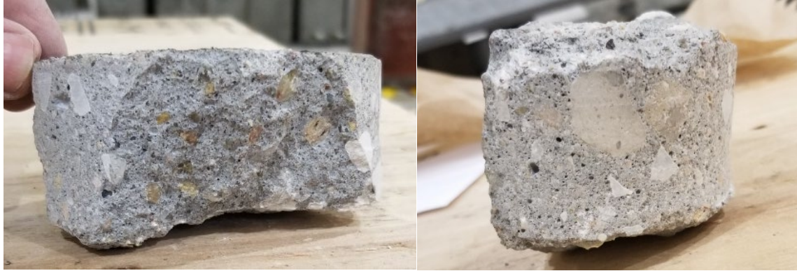
Figure 30. Extracted cores from the concrete specimen
