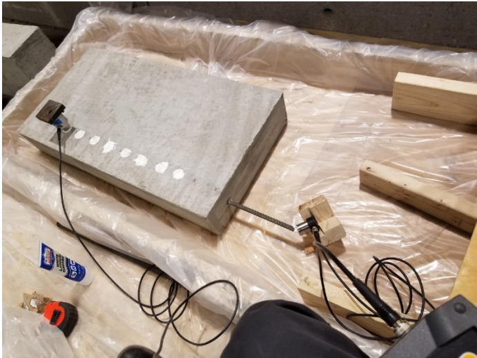
Figure 6. Experimental setup illustrated on one of the Specimen Set 3 slabs
