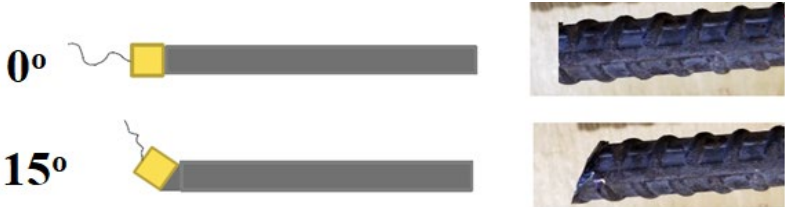
Figure 36. Bar end angles for corrosion specimens in Specimen Set 3
