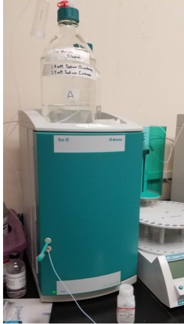
Figure 32. Eco IC Chromatography System from Metrohm
