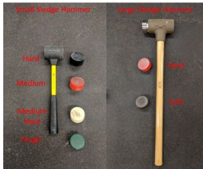
Figure 10: Different hammers and tips used for testing
