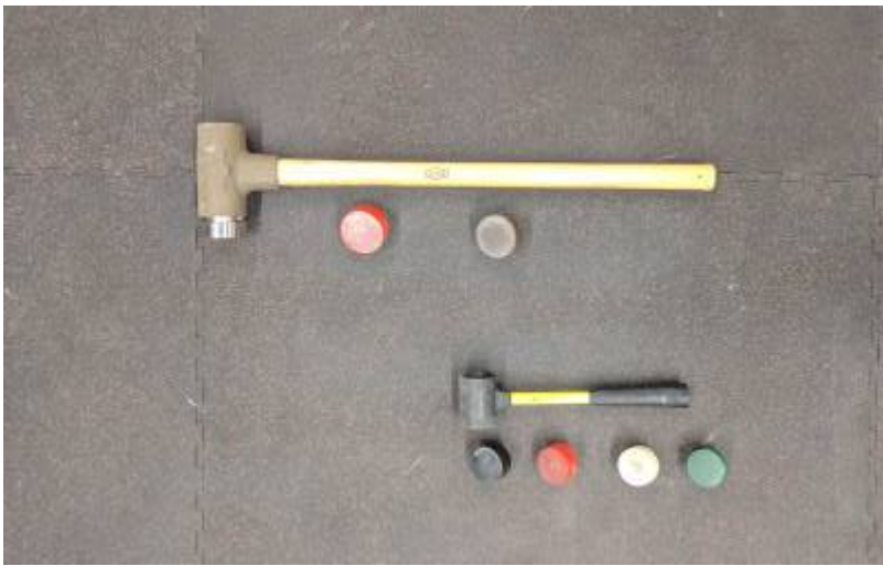
Figure 56: Different hammers used for testing
