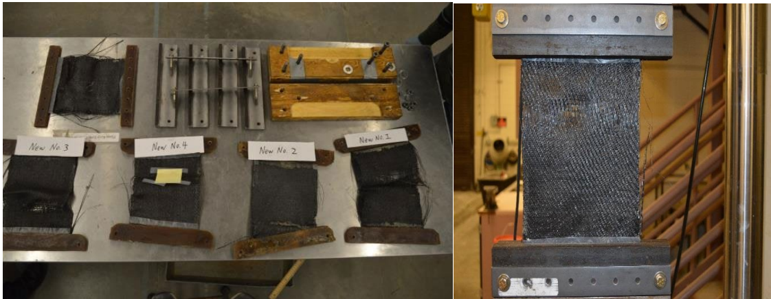
Figure 25. Wide width tension test sample preparation parts and layout
