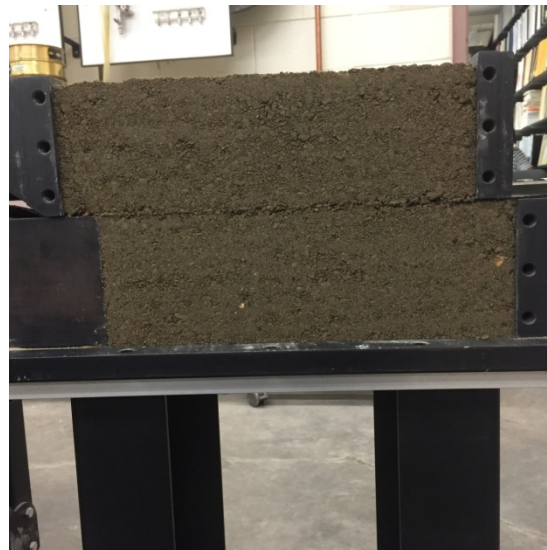
Figure 46. Backfill with geosynthetic inclusion after shearing
