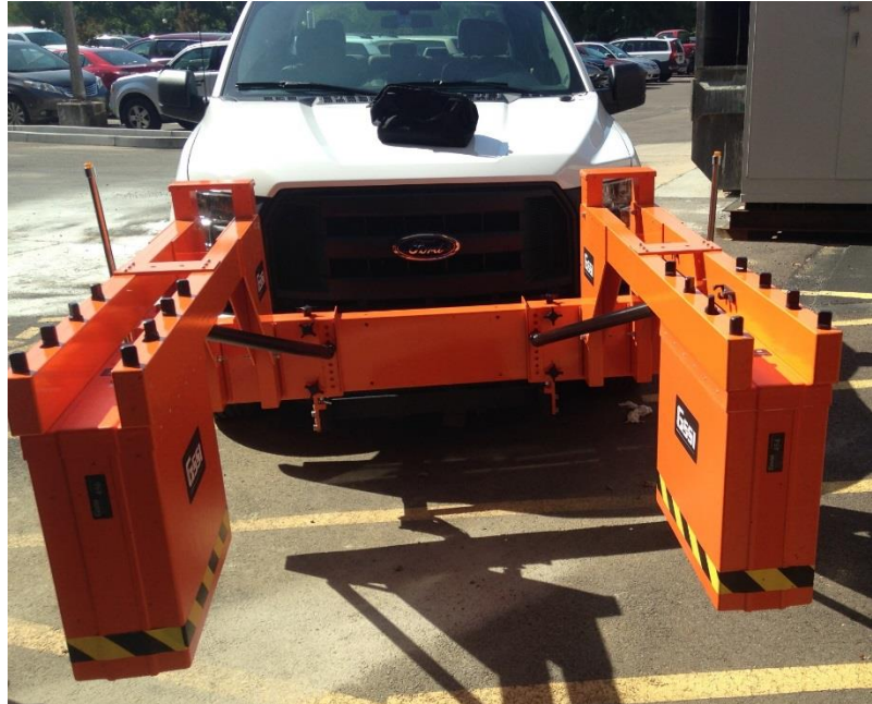
Figure 4: Picture of the antennas setup in the wheel path configuration.
