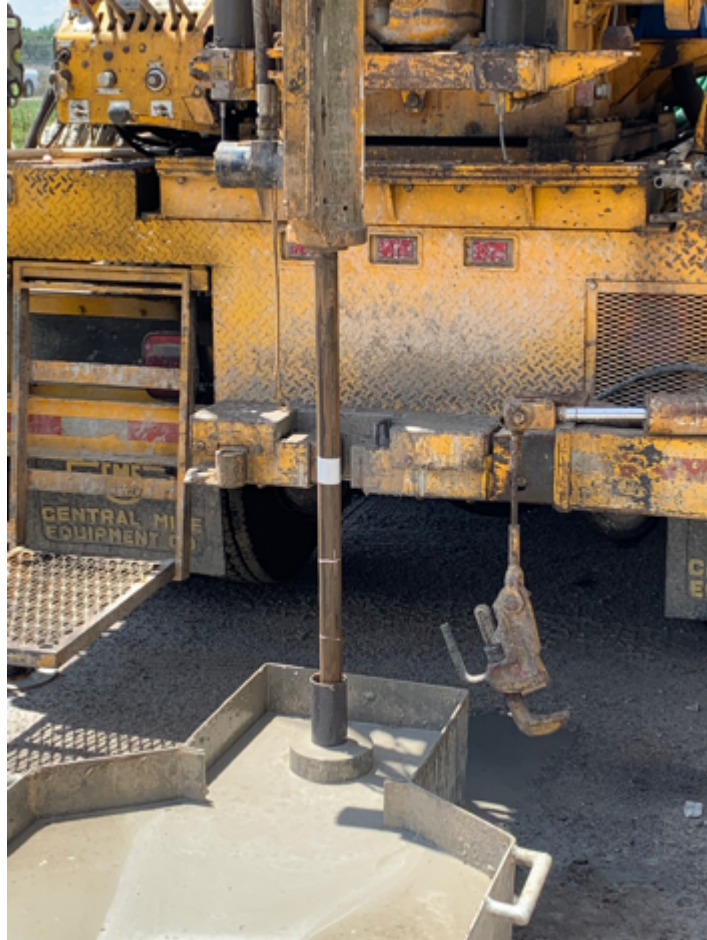
Figure D-4 Typical CMS and PDM SPT Rod Markings
