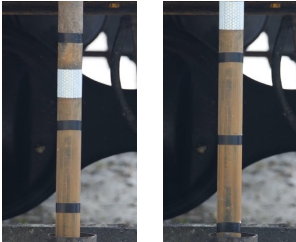
Figure 6-32 Dunns Creek SPT Rods with White PDM Reflective Tape and Black CMS Tape
