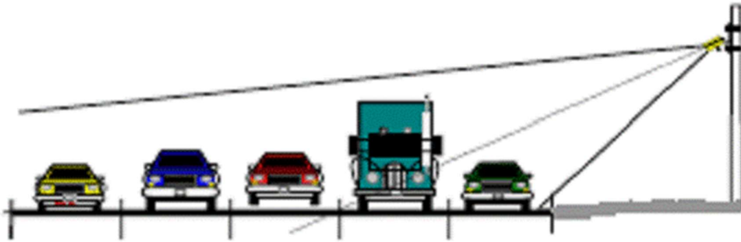
Figure II-1 Side-mounted configuration of RTMS
