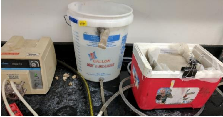
Figure 4.2 Horizontal flow permeability test
