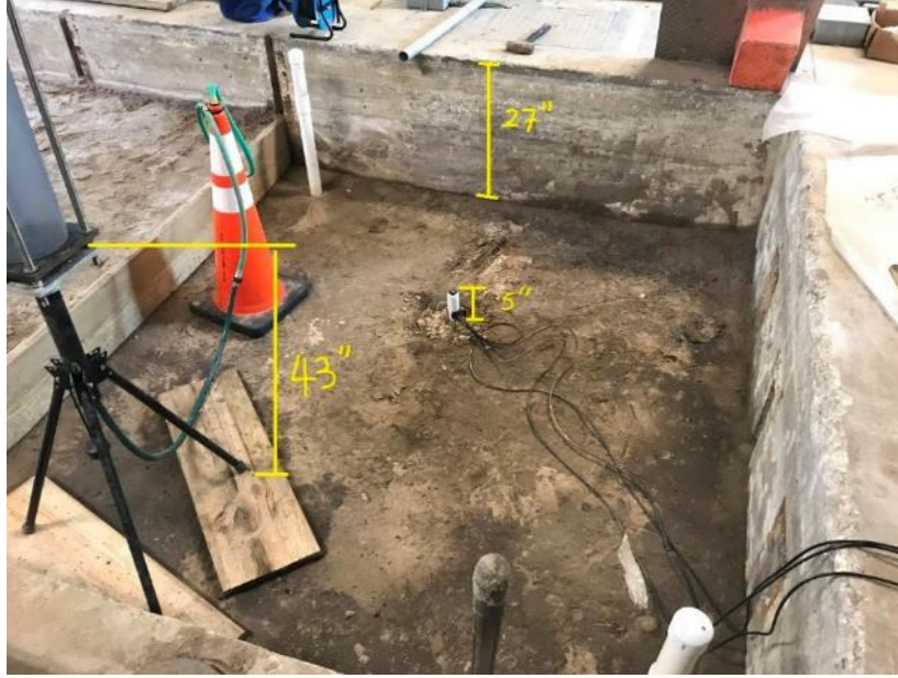
Figure 5.2 The setup of test pit at the FDOT State Materials Office using the PVC prototype
