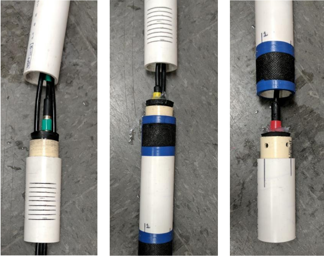
Figure 3.12 Upper, middle, and bottom chamber (from left to right)
