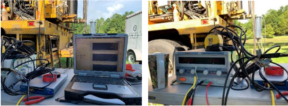
Figure 6.9 VAHIP Labview Program with power supply setup in field
