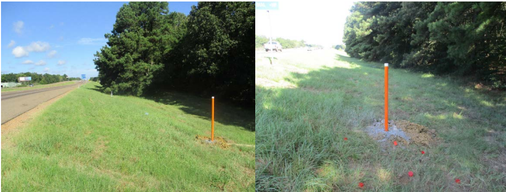
Figure 4.60 Slope 6 slope inclinometer installation
