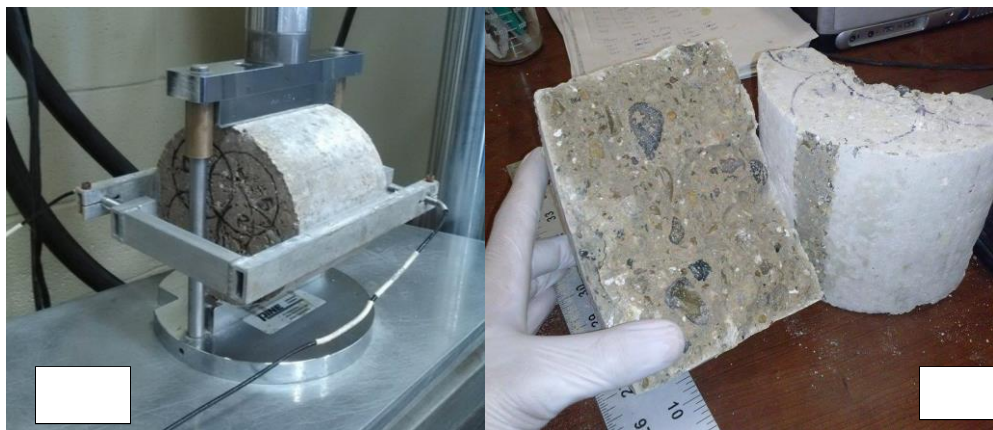
Figure 5.31 – Dynamic Indirect Diametrical Test (IDT) (a) Specimen Setup (b) Fractured Specimen
