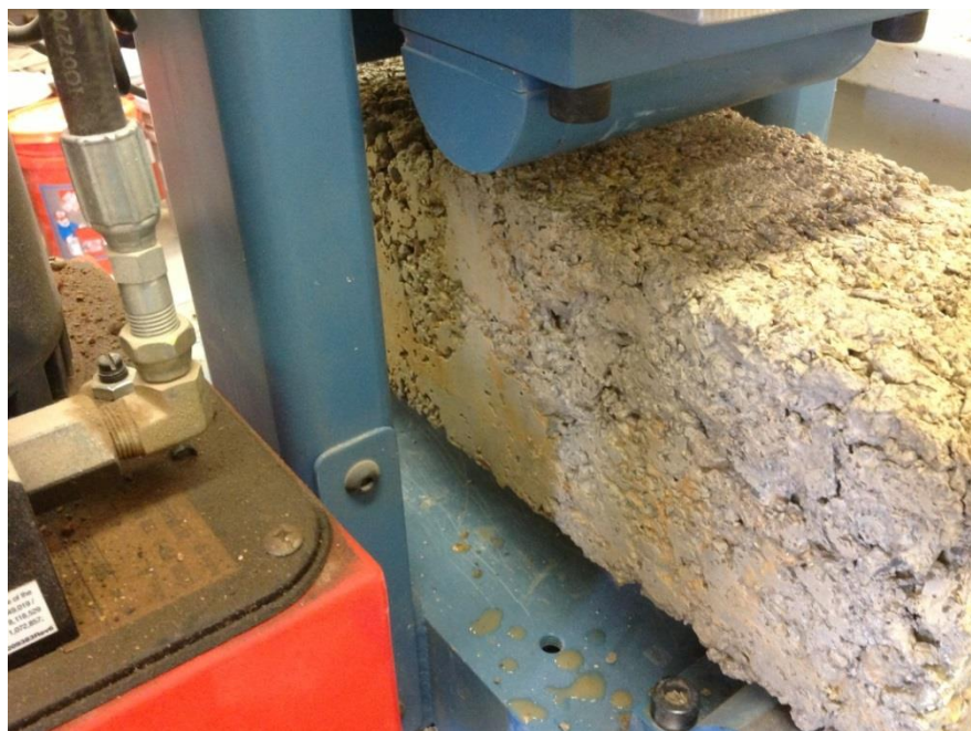
Figure 2.2 – Large Beam Fatigue Test Setup before Loading at UTEP
