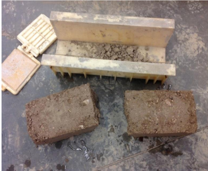
Figure 2.1 – Sample Breakage during Demolding and curing at the CTIS Laboratory
