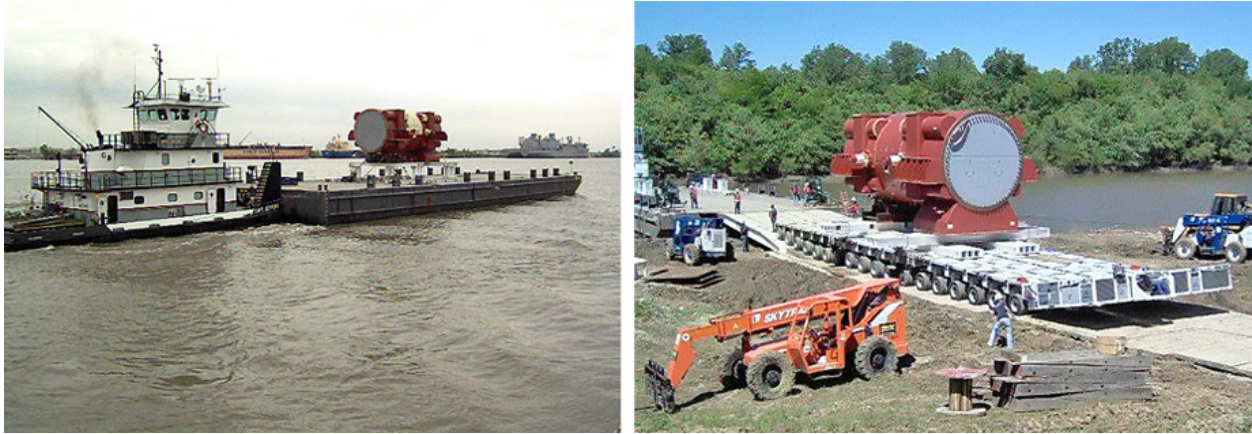
Figure 1: 250 Ton Nuclear Steam Generator Moving on a Special Flatcar after Unloading from a Deck Barge
