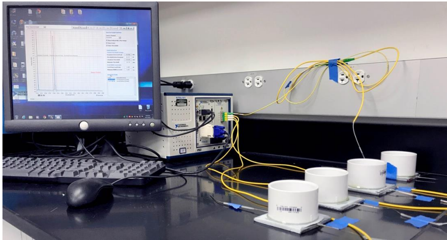
Figure 58. Integrated system in accelerated corrosion test setup.
