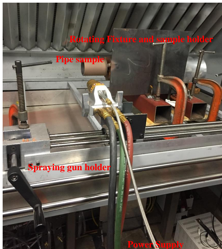
Figure 5. Automatic rotational fixture for pipe samples.
