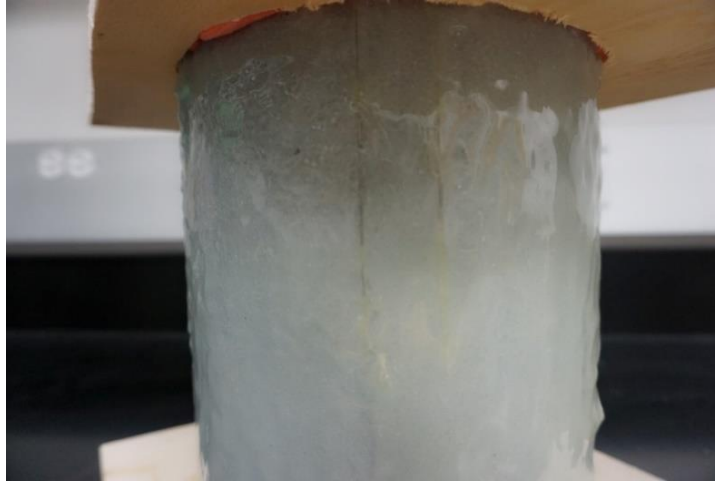
Figure 94. Pipe samples coated by multiple-layer coating with wire arc sprayed Al-Zn coating sealed by epoxy
