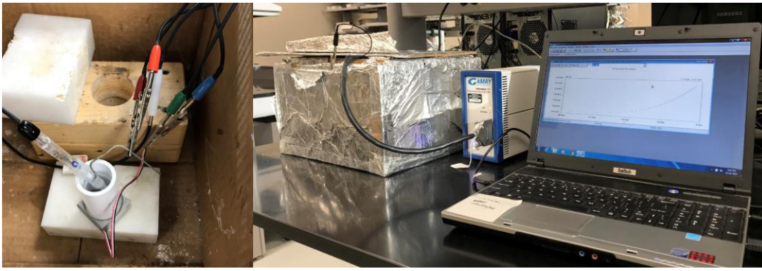
Figure 33. Accelerated electrochemical corrosion test setup.
