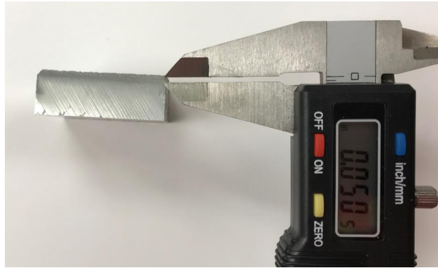
Figure 10. Measurement of coating thickness.
